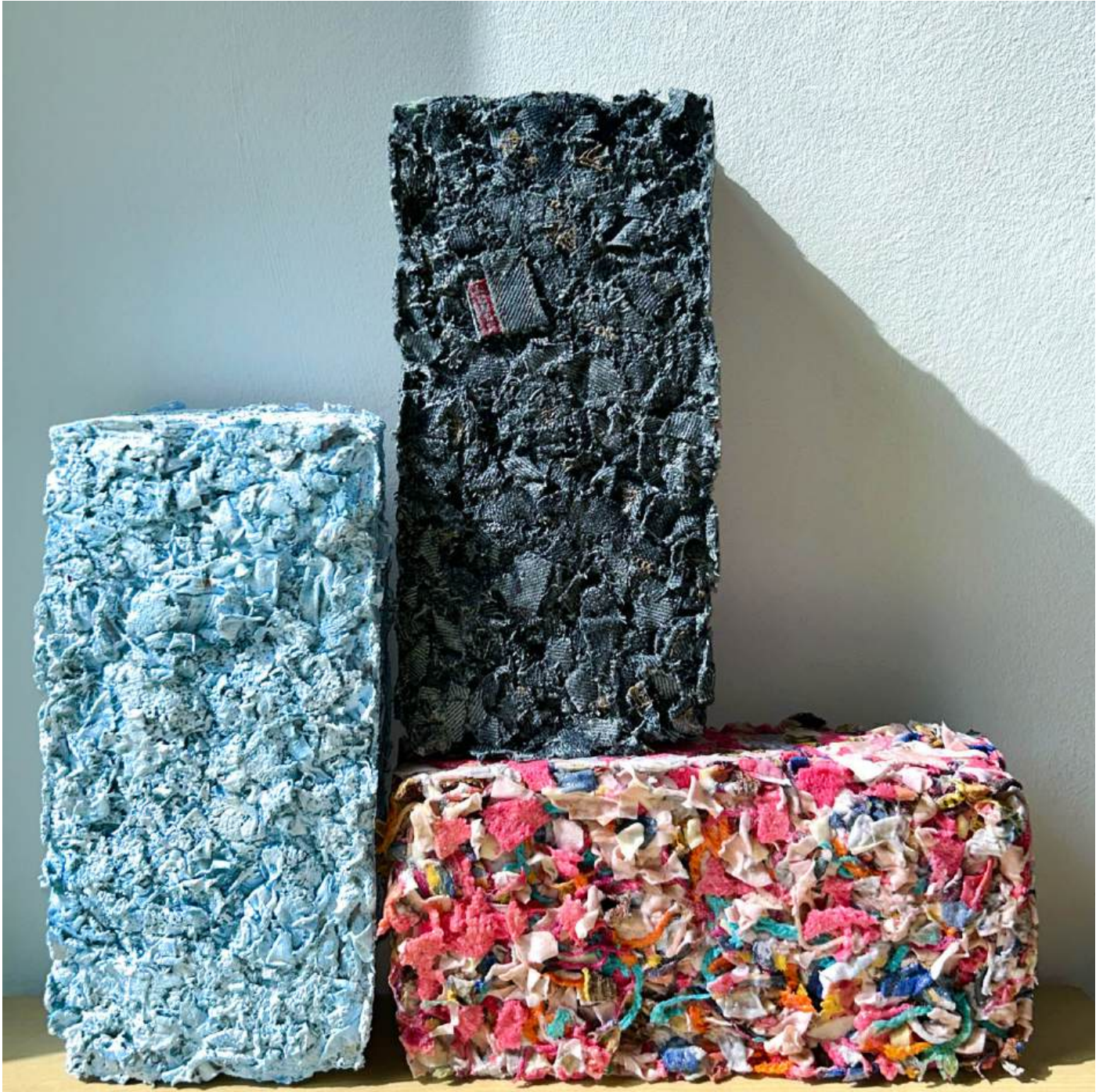
Bricks made from textile waste which have been compressed with glue into a mould. Experimenting with different materials, t-shirts, Towels and Denim to create different effects.
