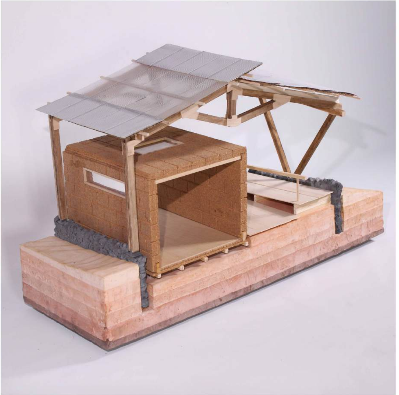
1:20 Section Model - Canopy Structure and Interior Cork Spaces
