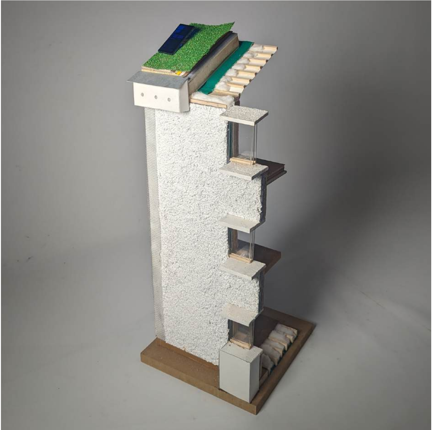
A proposed sectional detail model (1:20 scale) of a housing unit in South Manchester addressing comprehensive retrofitting, embodied carbon and biodiversity enhancement.
