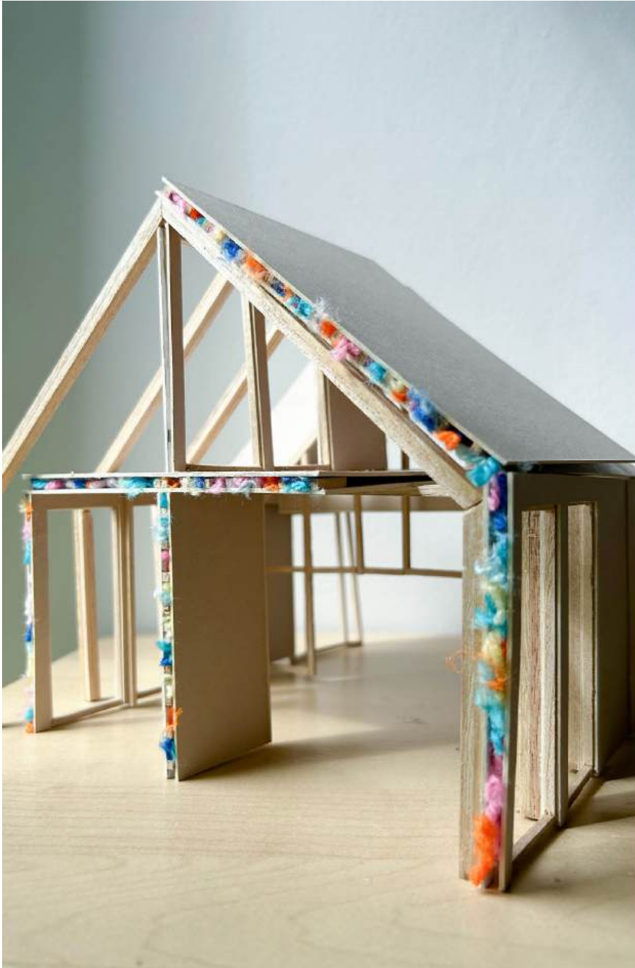
1:50 sectional model showing textile waste insulation and thermal envelope it creates. This model also shows the light pattern created from the skylight.
