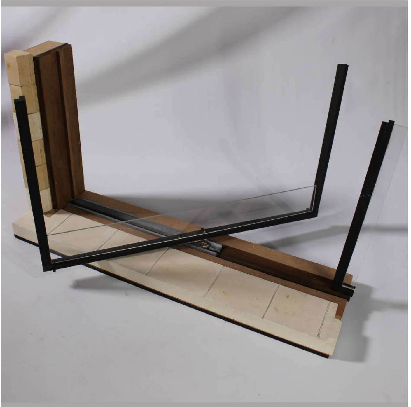
Image of my 1:5 ground floor detail showing how the buildings function can be changed depending open the weather through a functional model.
