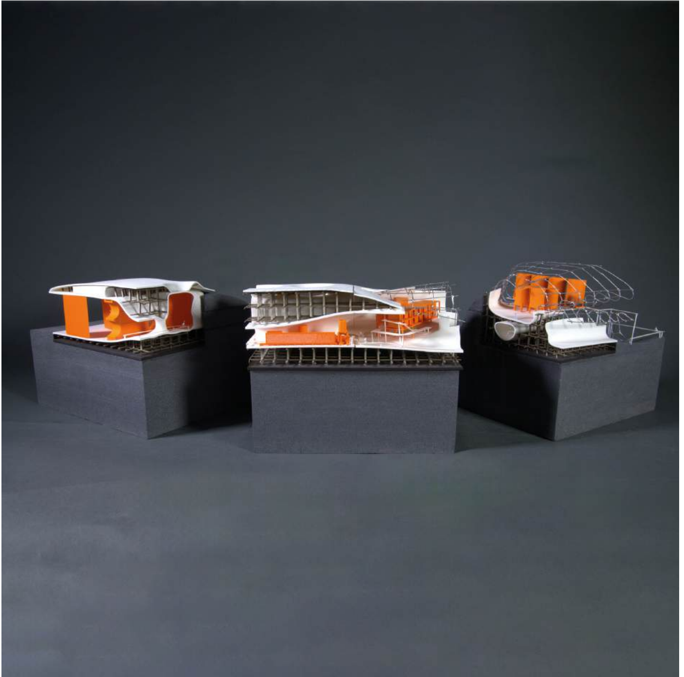
Interactive Model in which the different sections are pulled apart. Showing the wind entry section on the left, the main process area in the middle and the community and delivery are to the right.
