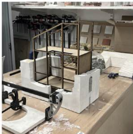
"Physical Model Two, Reusing the Pele Tower (Old Meets New), Studio Three. The picture illustrates the process from left to right, starting with the mold of the old building and the use of jasmonite for casting, followed by the cleaning of the cast and the addition of the new MDF structure."
