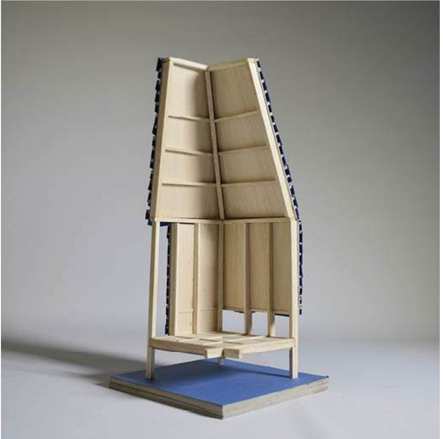
A corner detail model at 1-20 scale of a temporary exhibition pavilion demonstrating the relationship between the interior, exterior and the flood water level below. The model is clad in a plastic blue facade made from repurposed plastic.
