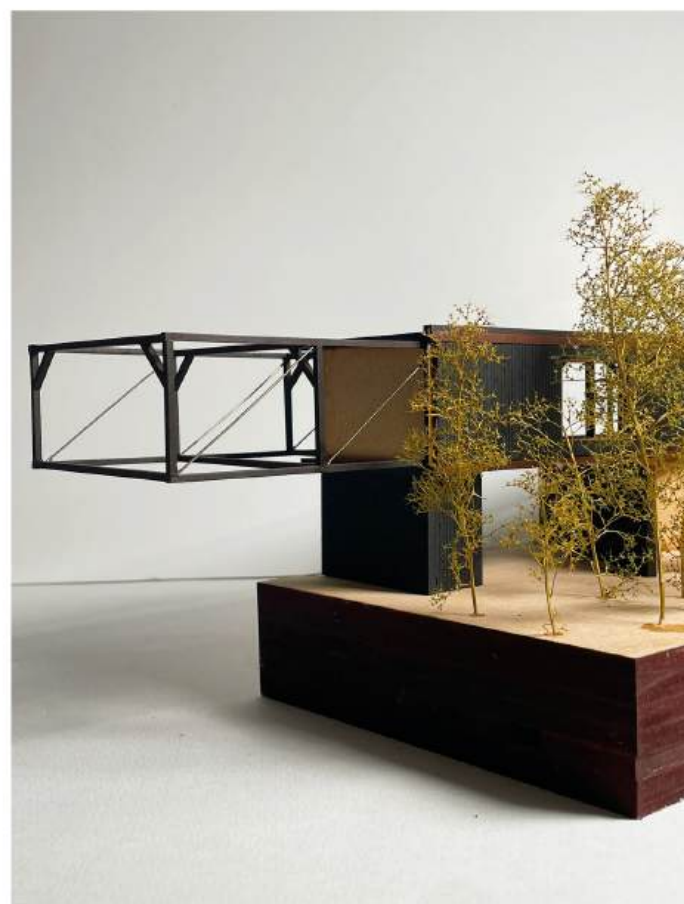
Cover Image B: View of the exposed structure of the cantilever revealing the bracing. "
