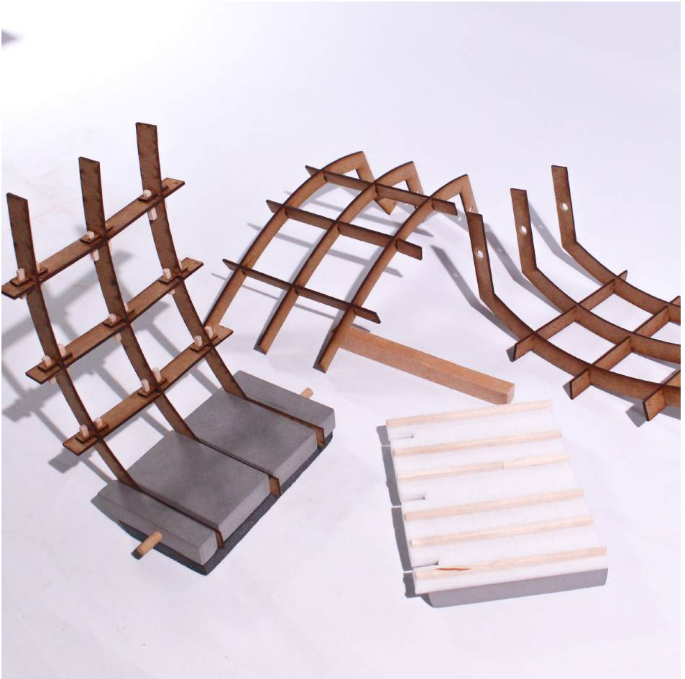
Fig. 3 1:20 Exploration of waffle structure joints
