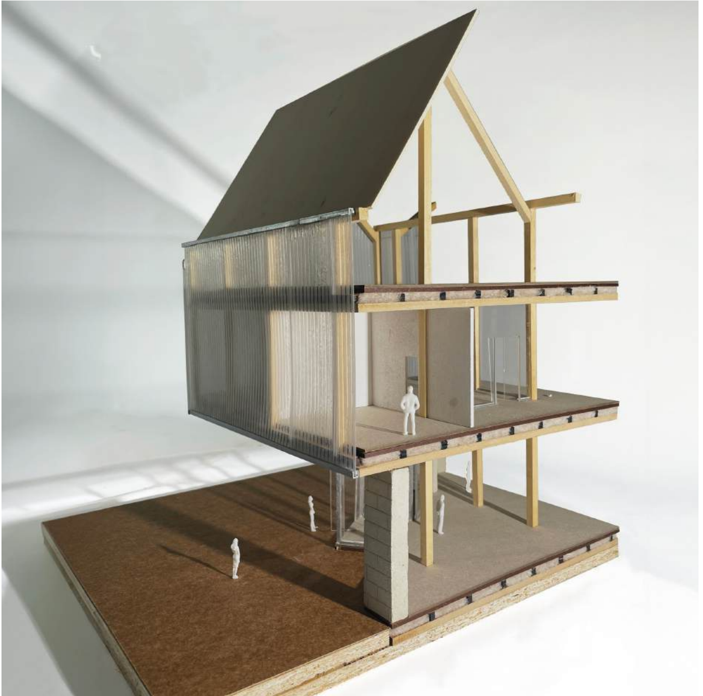
Final 1:50 corner model illustrating the section cut and the relationship between the interior and exterior spaces of the chosen corner. The structural strategy of the facade and floor build up is visible with indication of some interior spaces.
