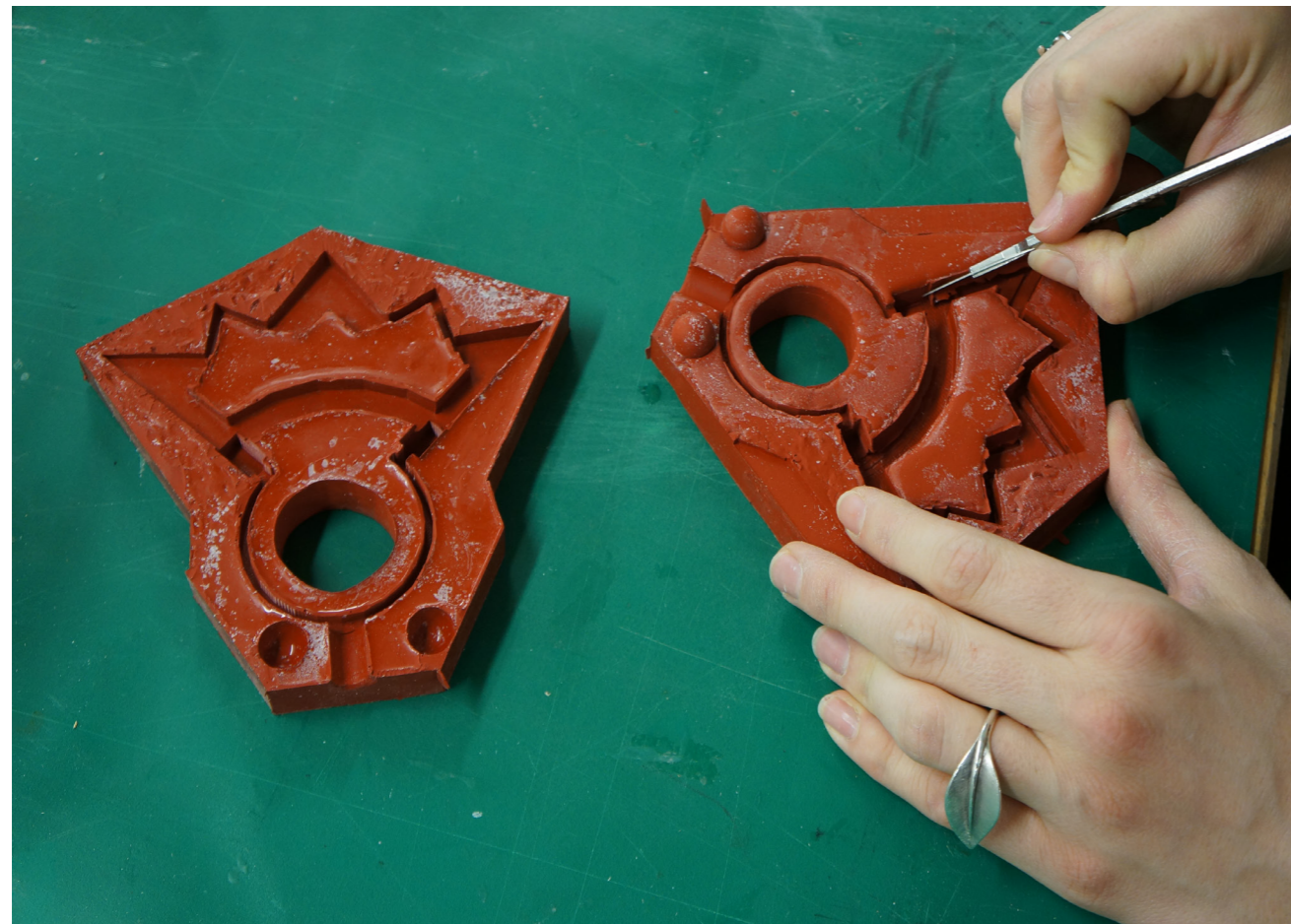
1: 10 detail fabrication using a silicone mould, by Jana Kefurtova
