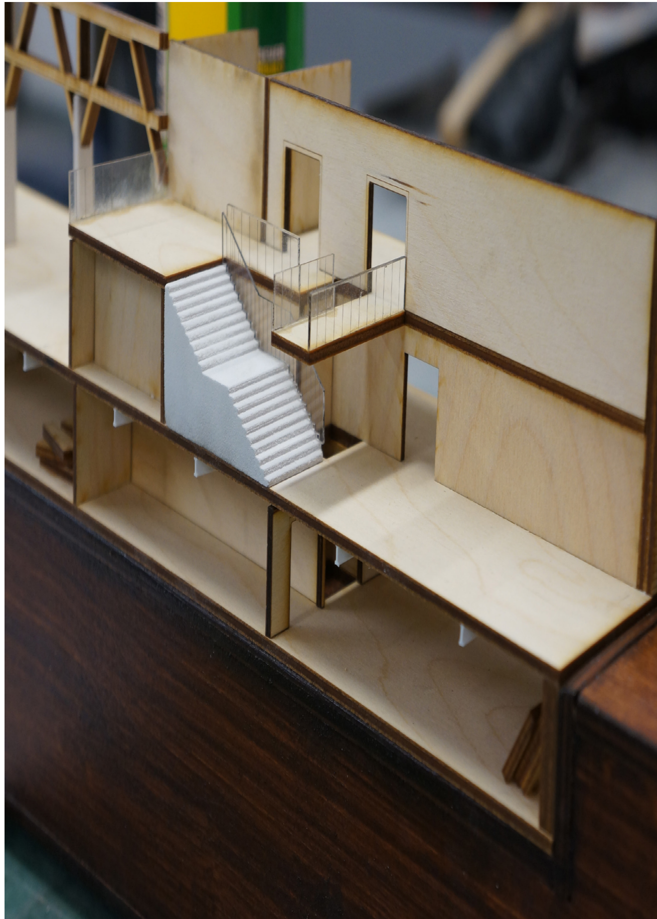
1: 100 sectional model using etched 3mm plywood, by Daniel Kempski
