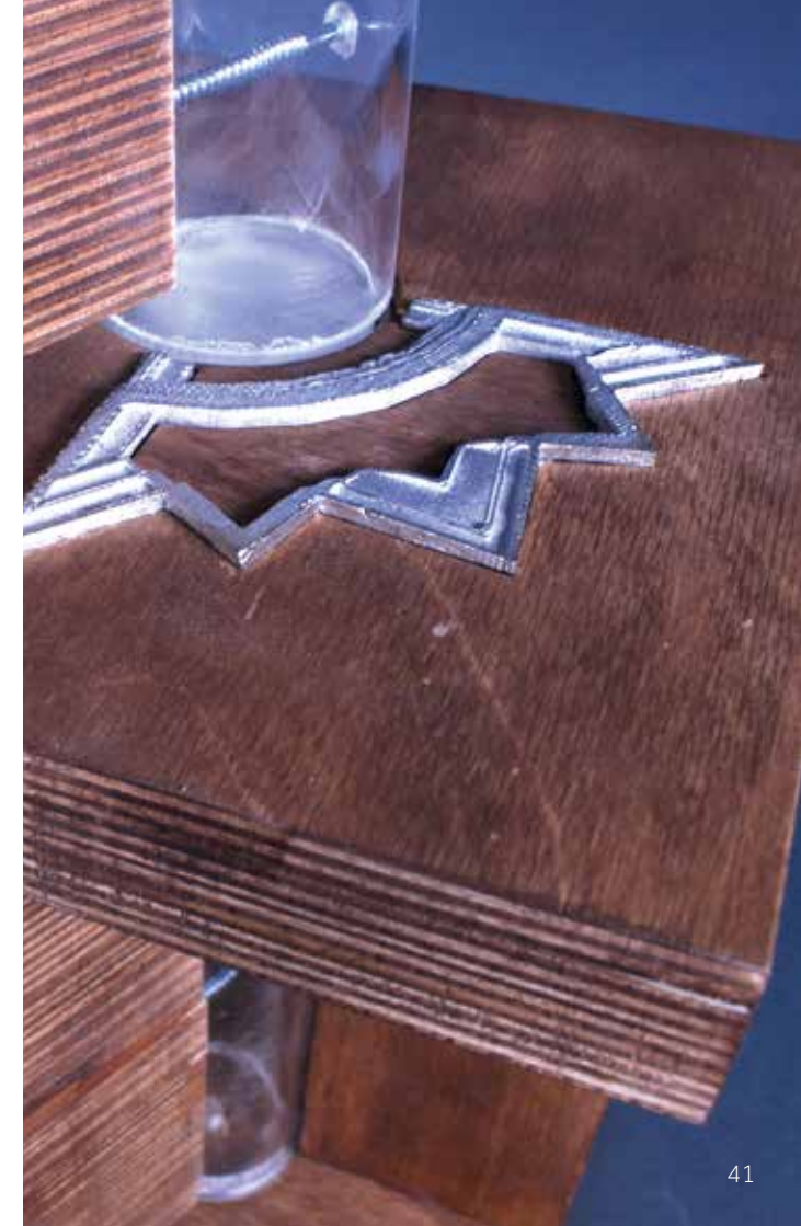
'HOME TRACKS BREWING HALL' BEER PUMP PROTOTYPE Monty Dobney, 2016 This 1:1 prototype was designed with continuation of the running ring pattern theme that Monty established earlier in his project. The model uses ABS 3D Printing, Copper Pipe, Copper Metal Powder cast into Polyurethane Resin and Laser Engraving on the wooden tap handle. Other models from this series are visible in case 4 and case 7.
