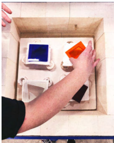
Image 04: before slumping The kiln allows it to warp within the parameters of the template. The forms take shape of the participant's location plan.
