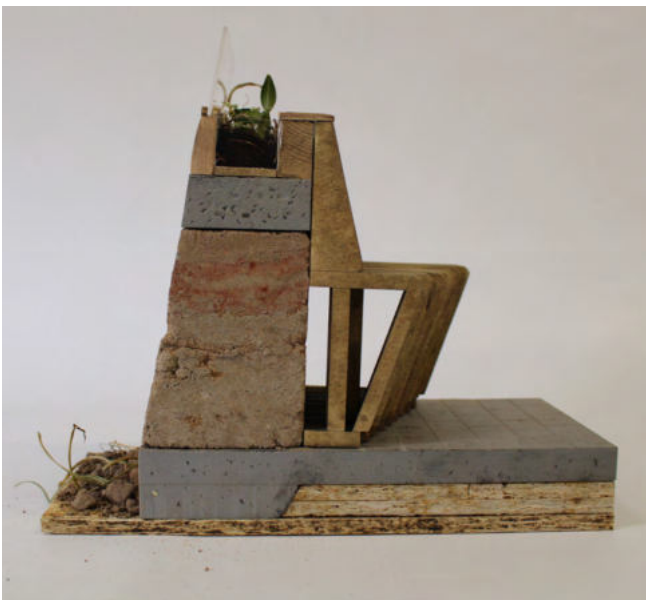
Image 01: Surface for Rest: 1:5 model section view Materiality: Timber, concrete, earth, glass, and planting
