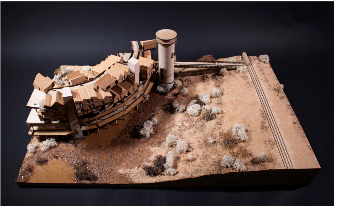
Image 01: Photo of 1:200 sectional model demonstrating scheme interaction with topography, wetland and tram access. Created using MDF, plywood, cork, plaster, wood glue and epoxy resin for the habitat texture and wetland.
