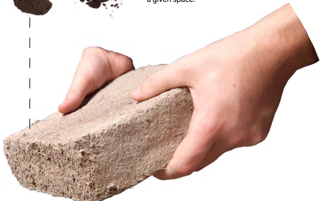
Image 02: Standard Glass-Earth Brick 200mmx200mmx70mm - These dimensions were selected to accommodate both single and double leaf masonry, based on U-Value requirements for a given space.
