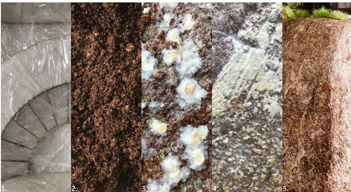
Image 06: Mycelium base process. 1. greyboard mold built according to existing gasholder water chamber dimensions; 2. sawdust & coffee ground substrate mixed with oyster mushroom mycelium spawn; 3. mycelium allowed to grow over two weeks; 4. mold removed; 5. base dried to kill off mycelium.
