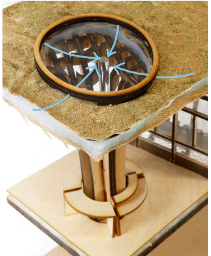
Image 04: Clear acrylic rod as transparent drainpipe in the centre of column; rainwater runs down to lake through here (drawn in blue) entering from gaps in between louvres around the raised skylight, visible to users
