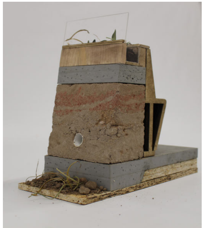
Image 02: Surface for Rest: Rammed earth wall exterior view
