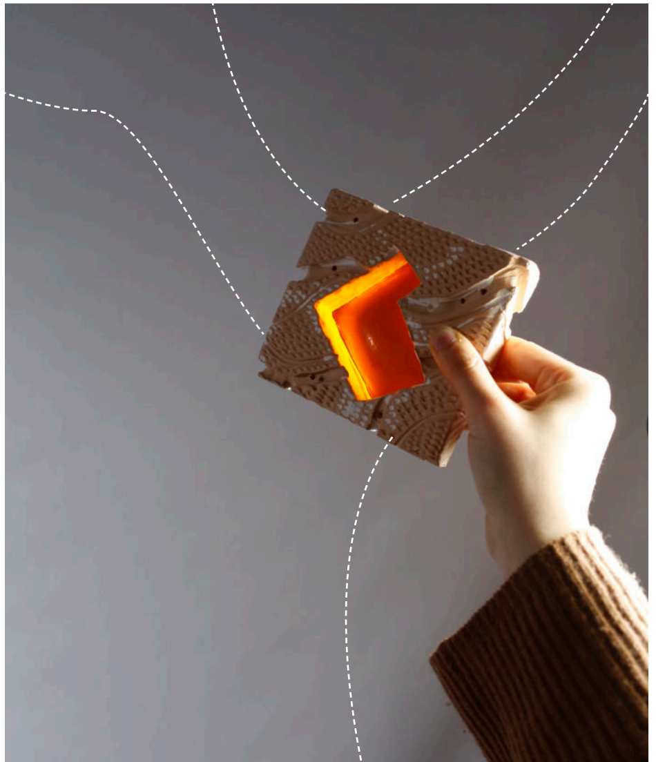
Image 06: developmental 1:1 segment of my proposed stoneware ceramic panel finished with embedded coloured slumped glass. A series of these panels show a facade mapping of Iraqis all over the world.
