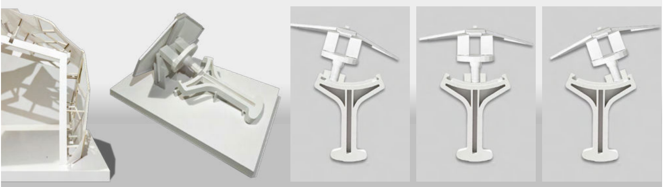
Image 05: Sectional Construction Model 1:50 & Adjustable Y-Mullion + T-Bracket Jointing Model 1:1
