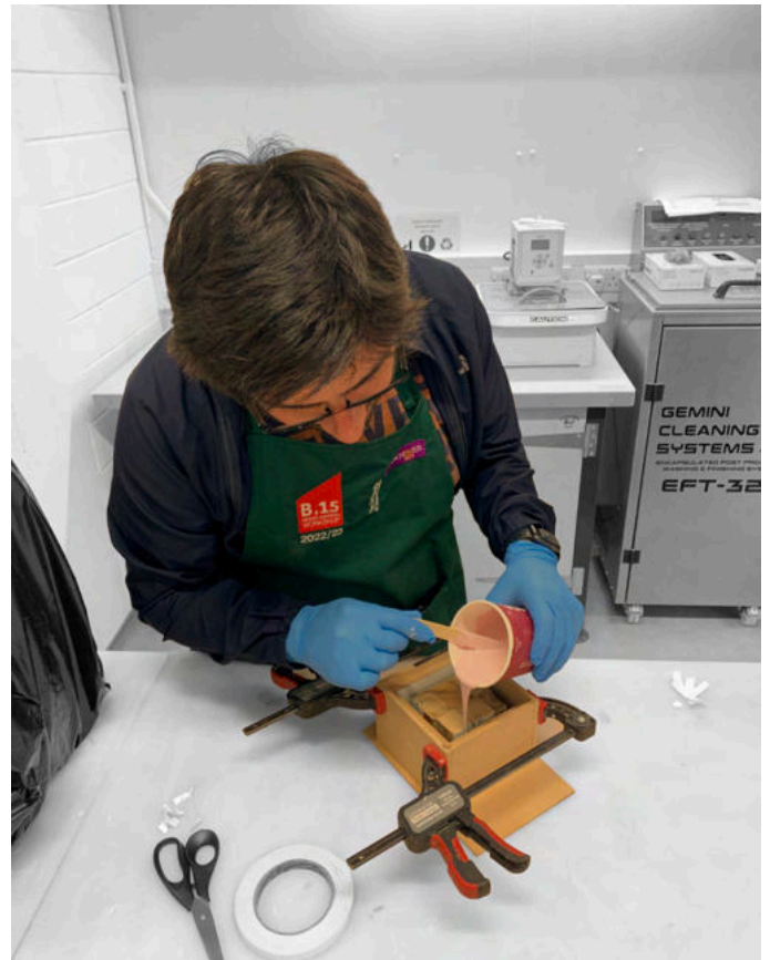
Image 02: Casting silicone molds for resin
