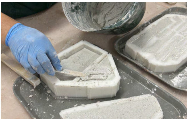
Image 05: Making Process - The plaster is mixed in proportions and poured into a mould made by silicone.
