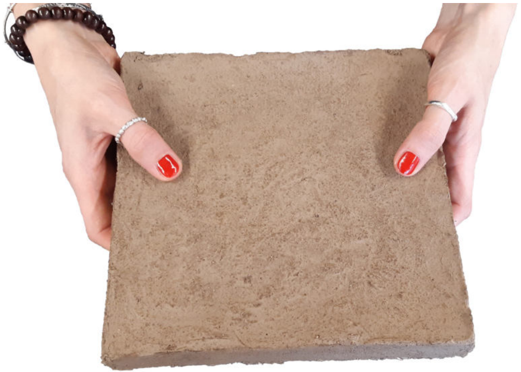
Image 03: Thin Glass-Earth Brick, 200mmx200mmx30mm, can be laid as a pair with 10mm mortar between to match the standard brick.
