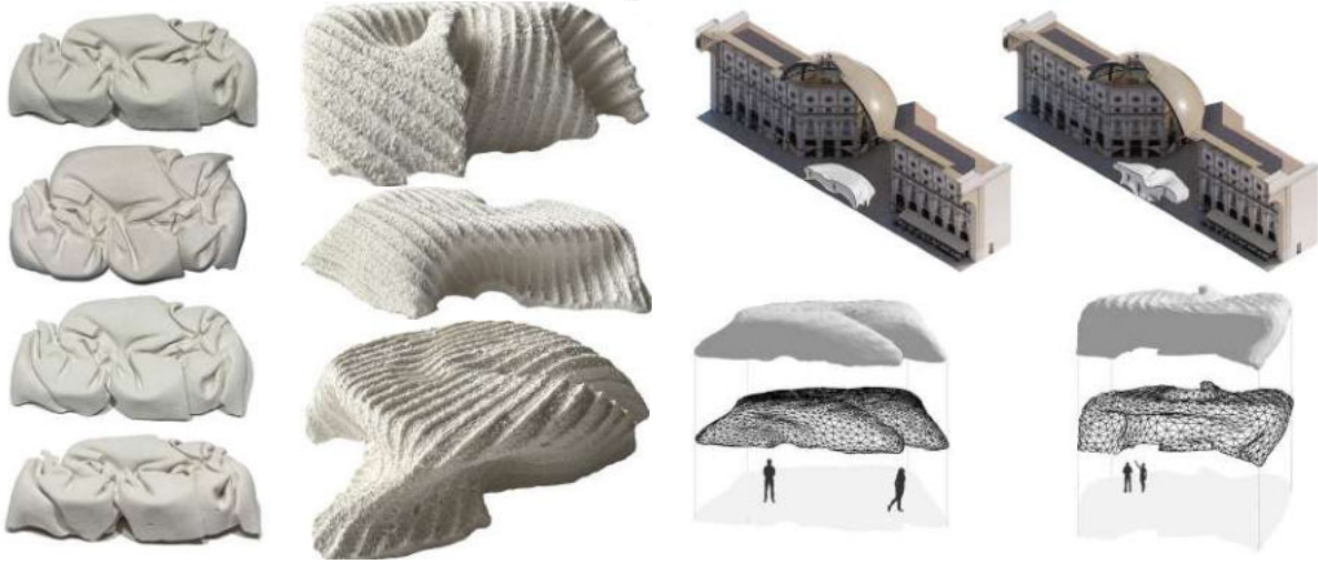
IMAGE 03: Casting plaster in fabric, created individual unique peices that then informed the shape for a pavillion
