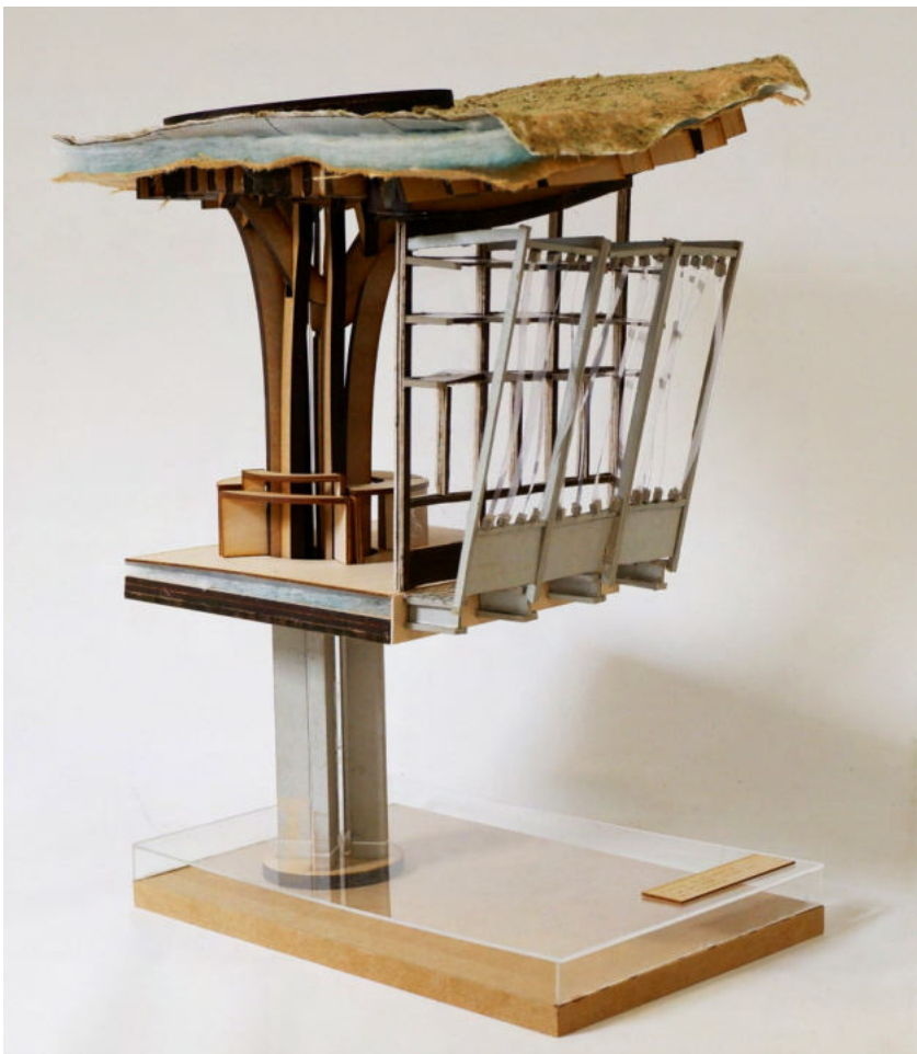
Image 01: Finished 1:20 bay model exploring the complex relationship between the column, roof, and double skin facade
