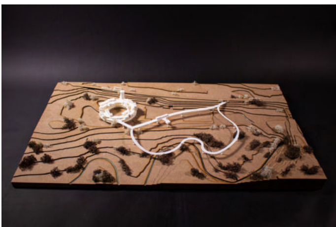
Image 05: 1:1000 Site model demonstrating the promenade route throughout site and scheme interaction with non-human habitats (wetland, scrub and woodland). Created using layered MDF with 3D-printed elements.
