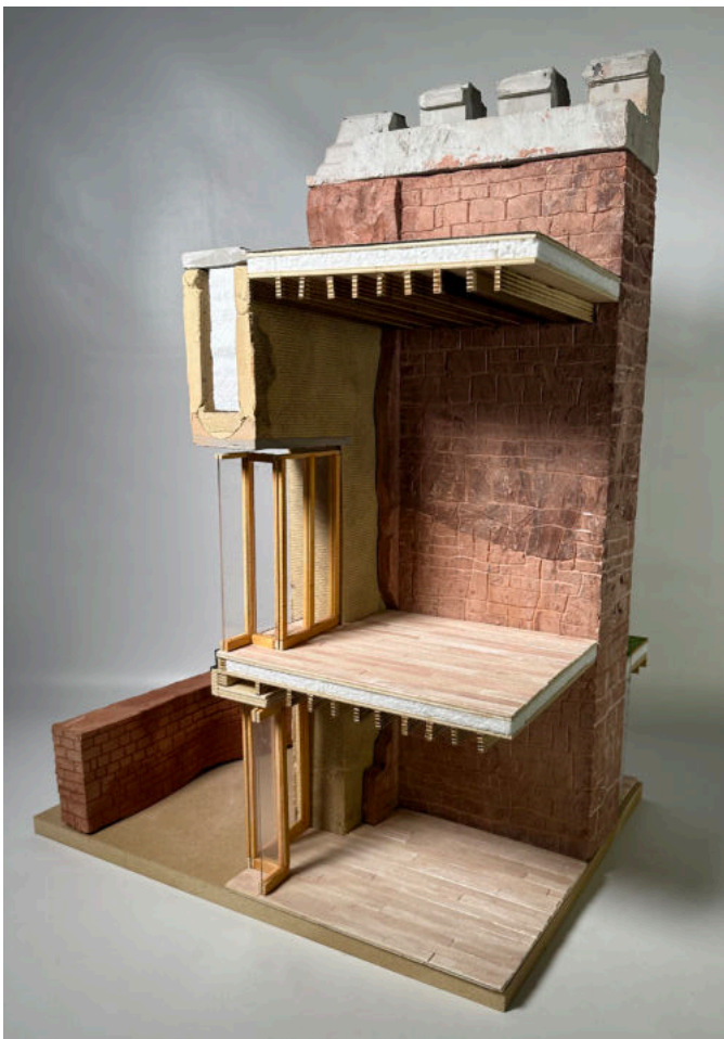
Image 05: Internal view illustrating how the new joinery element meets the existing stonework
