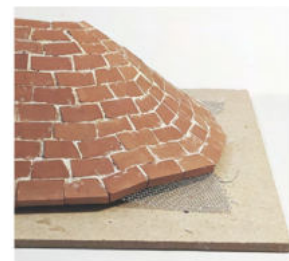
Image 06: Experimenting and testing funicular forms using terracota bricks
