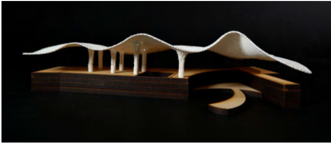
Image 02: 1:200 model showing form of roof (3D printed ABS) in relation to plan (engraved with laser cutter on MDF)
