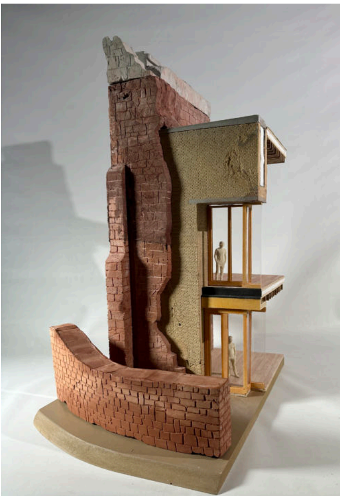
Image 01: 1:20 sectional model that demonstrates the 3 main elements of the building: Existing stonework, new joinery and brickwork
