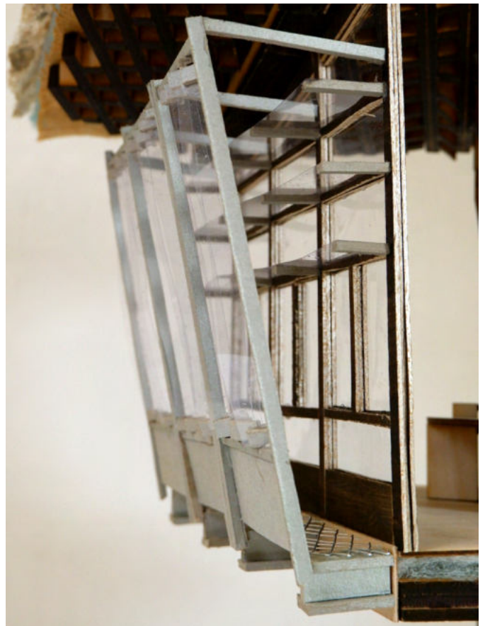
Image 06: Double skin facade made by hand - Inner curtain wall: acetate and balsa wood - Outer panels: acetate and silver spray-painted greyboard - Grating: wire mesh on silver spray-painted greyboard
