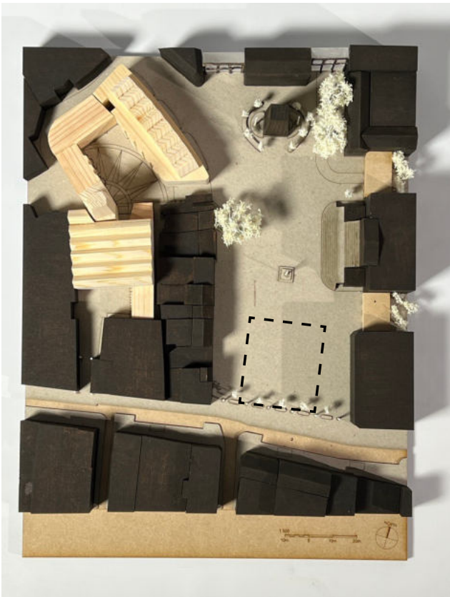
Image 01 1:500 Massing Model : Exploring the relationship of the scheme with the immediate site that is the Preston flag market, solid and void study. Dotted line indicates the tower block that was
