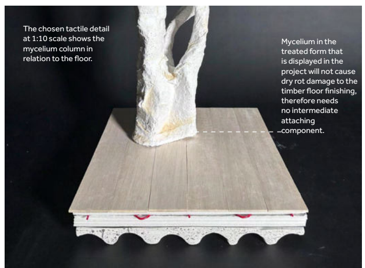
Image 03: Column was attached with cyanoacrylate glue
