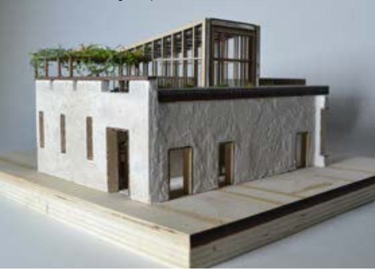
1:50 sectional model : Engraved plaster board and wall filler wall finishes.
