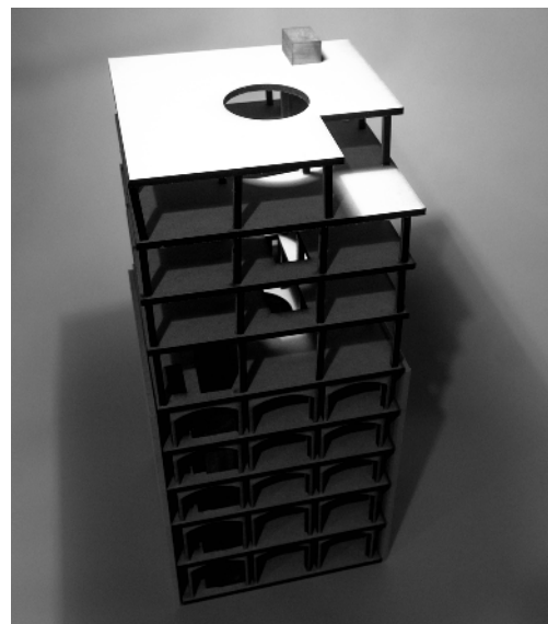
1:100 structural model exploring the chasm that penetrates the building.
