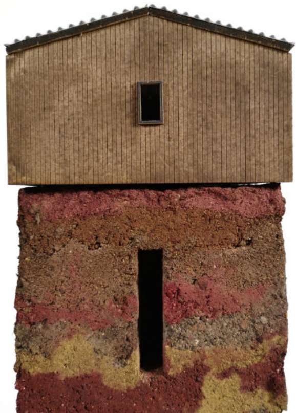
Image 01 + 02: "Seed Bank", 1:50 Rammed Earth models, hand rammed models made from 7 part soil and 3 part concrete. Acrylic paint added for pigmental differentiation. Existing elevated shed made from etched and stained mdf and corrugated card
