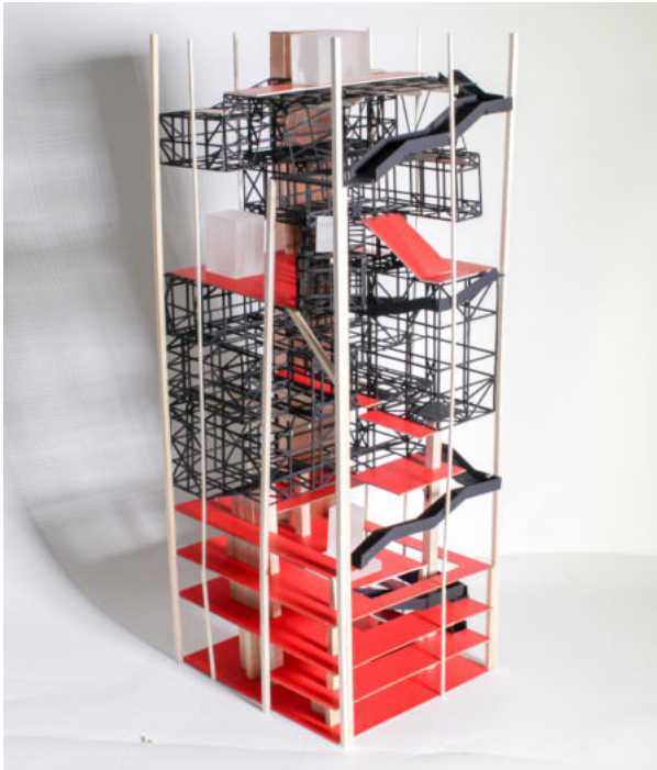
Image 3: Diagrammatic developmental 1:100 structural model -the relationship between structure and programme. (Made from coloured mountboard and Balsa wood)
