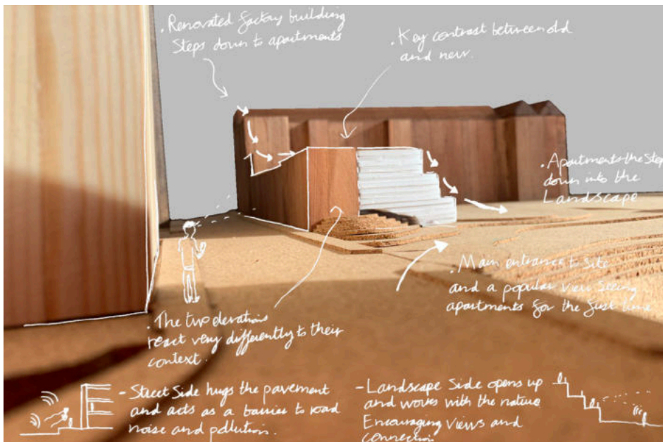
Image 02: Sketch massing model Mountboard with site model timber and cork
