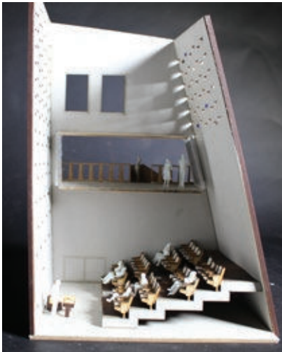
Image 04: 1:50 theatre space model expressing the vast perforated brick covered nodes & the connection between spaces: wood, greyboard, perspex
