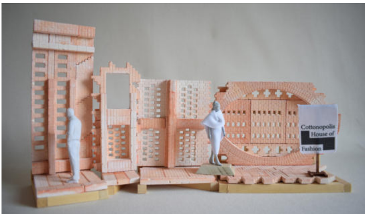
Image 04: 1:20 Materiality Tests - Plaster cast elements with jelutong framing.
