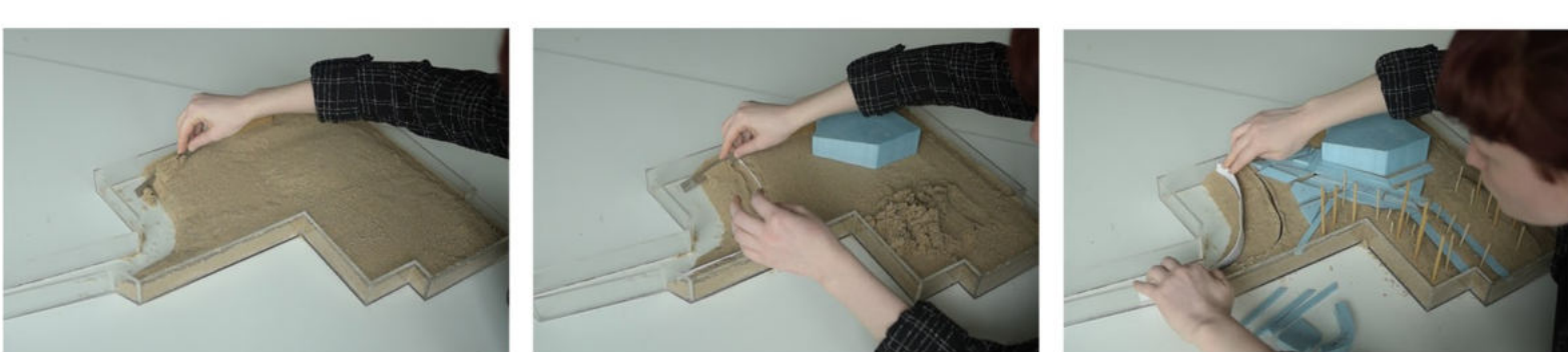
Image 04: Sandbox model with blue foam to represent hard landscape and plant beds and it was determined that this iteration involved too much intervention - 1:200.
