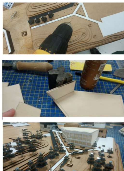
Image 02: Process of making the landscape model- drilling holes for nailed trees, fixing together complex angled pieces.
