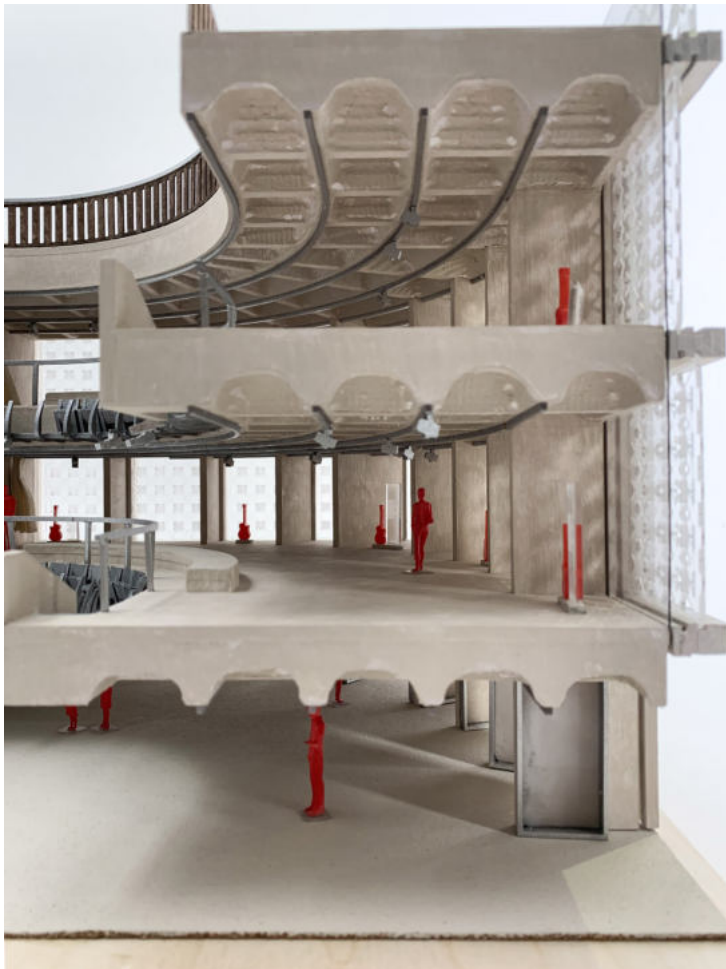
Image 01: Final 1:50 sectional model MDF, frosted/clear Acrylic & finished in acrylic & emulsion paint
