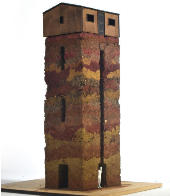
Image 01 + 02: "Seed Bank", 1:50 Rammed Earth models, hand rammed models made from 7 part soil and 3 part concrete. Acrylic paint added for pigmental differentiation. Existing elevated shed made from etched and stained mdf and corrugated card
