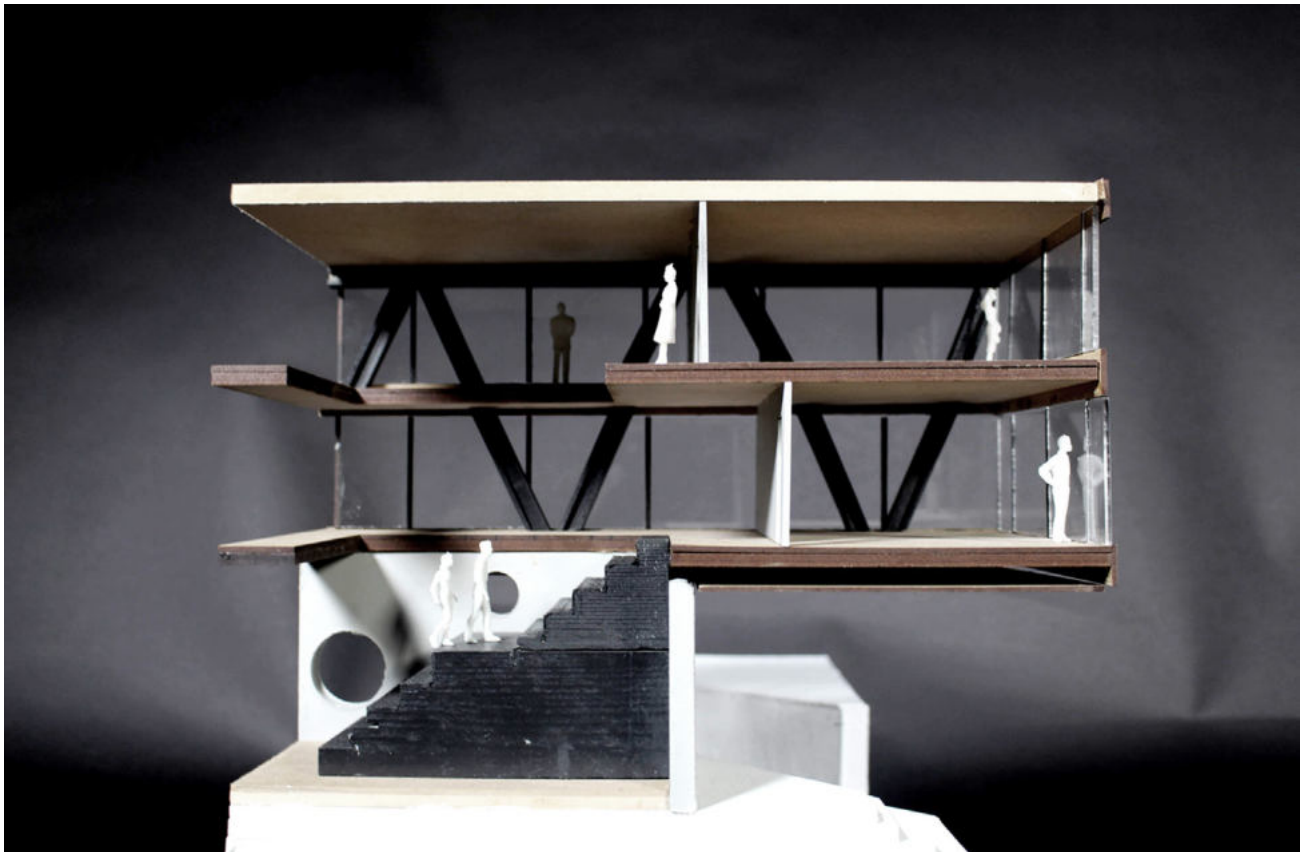
Image 05: 1:50 model of key corner in my building, the cantilever
