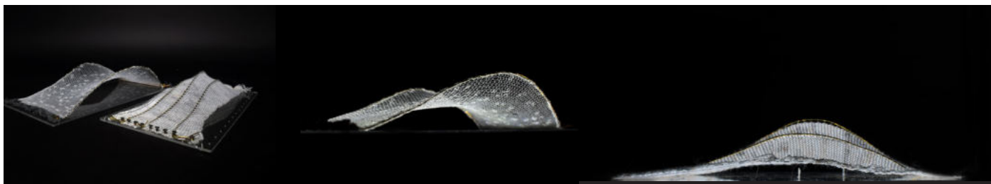
Image 03: Knit structure exploration via domestic knitting machine Clear acrylic, wire, mixed yarn
