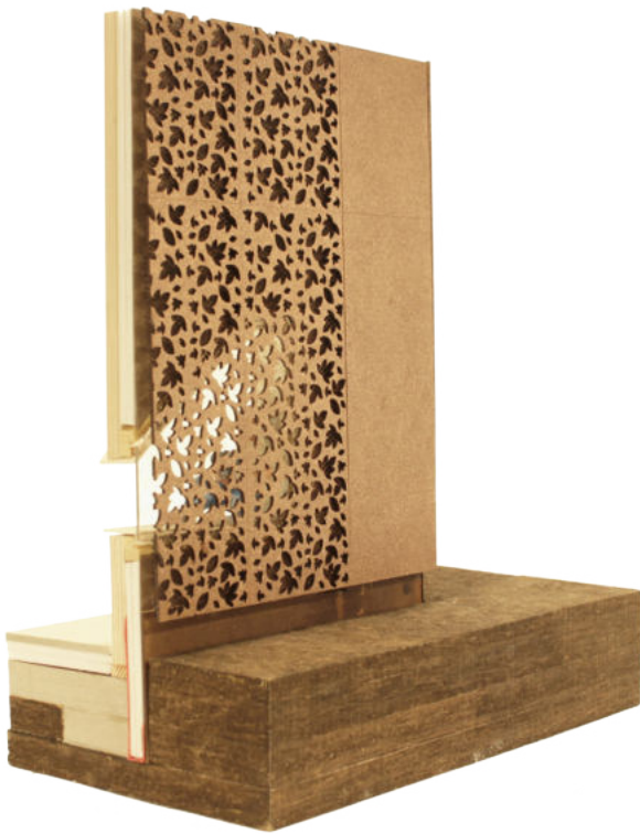
Image 06: Detail model- Wood, foamboard, greyboard, metal mesh, card, plasticine person
