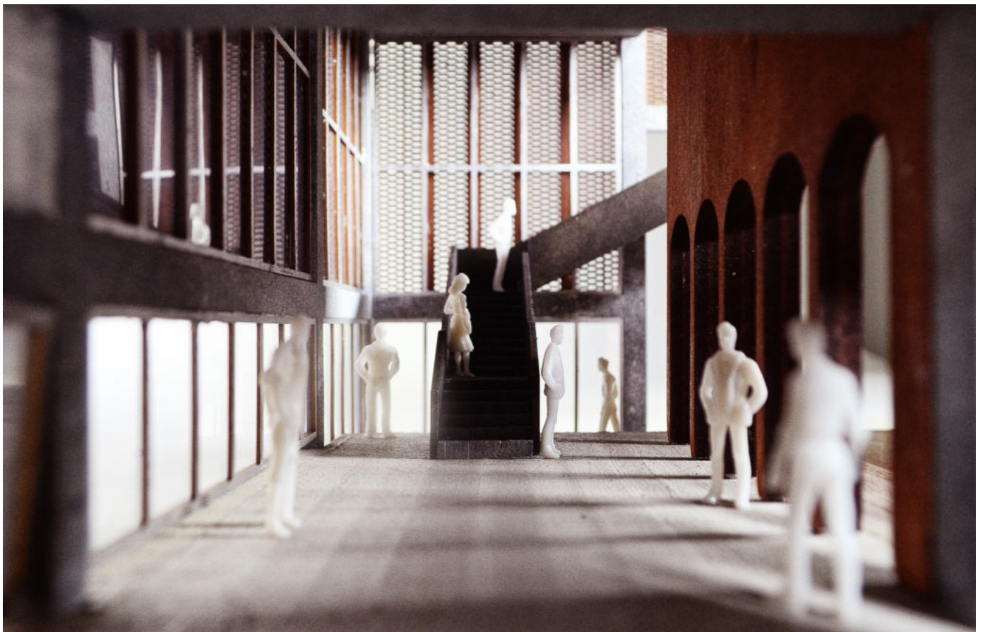
Image 01: 1:50 Internal Study Model MDF, Image transfer, Concrete Screed, Acetate, Greyboard
