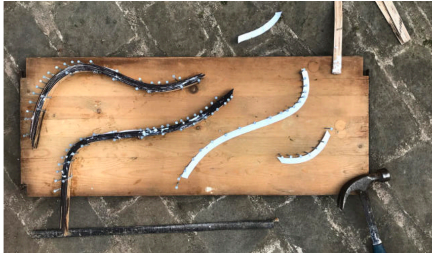
Image 2: Constructing the glulam beams. Six strips of ply curved around a set of nails with copious amounts of PVA and left to dry.
