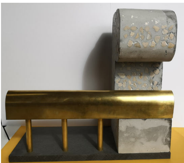
Image 06: 1:1 Handrail, Brass and Pigmented Plaster with Limestone Chips.
