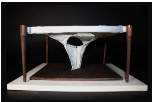
Image 01: Single surface, tensile fabric test Stained timber lathe-turned legs, Steel frame, hand-stitched fabric.
