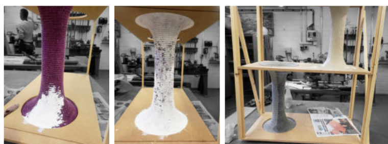
Image 06: Knitted formwork, structural cast Timber, knitted columns, cyanoacrylate, plasterboard adhesive
