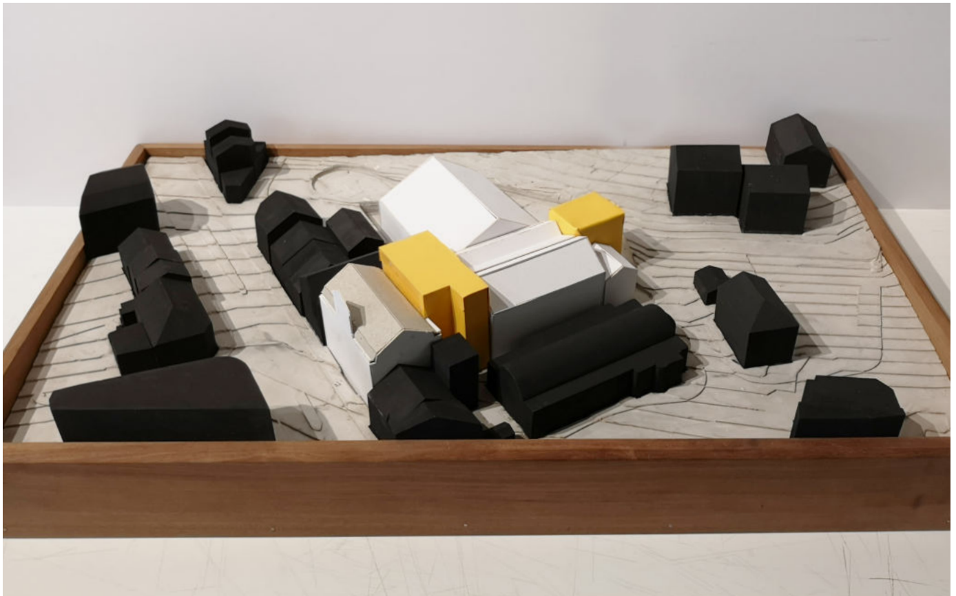
Image 01: Site Model, Pigmented Plaster and Stained Jelutong with Mount-board and Paper Insert.
