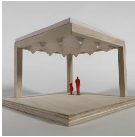
Image 03: Cast acoustic ceiling test Cast from 3D print in silicon mould, Beach wood, Ply
