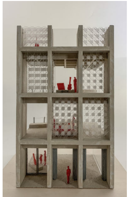
Image 06: 1:50 Facade Sectional model, Mdf, frosted/clear Acrylic & finished in acrylic & emulsion paint
