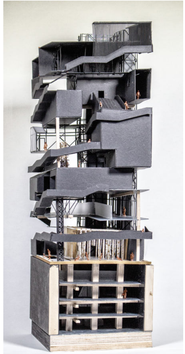
Image 4: Integration of refined programmatic and structural concepts into a 1:100 GA Model. (Made from Balsa wood, Acrylic, Plywood and laser cut mount board)
