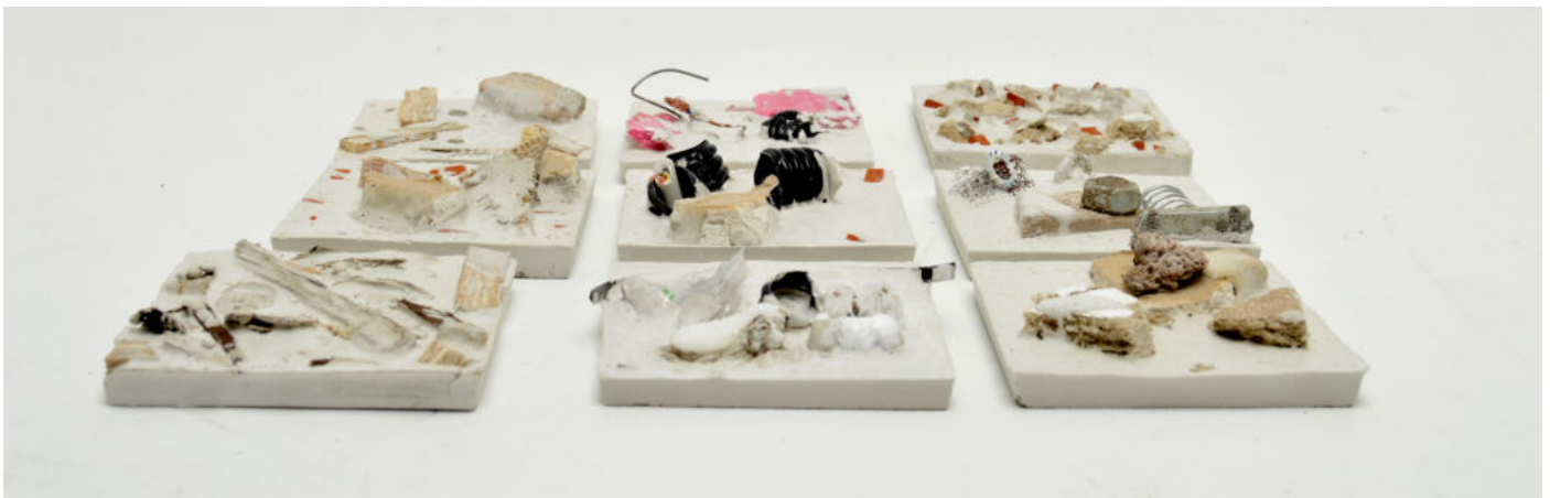
Image 14 (above): Material studies models Construction waste collected from UOM construction site, sorted and cast in a plaster cement mixture in a vaccum fomed mould)
