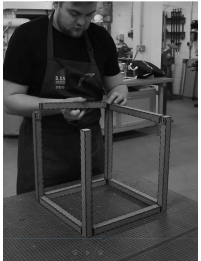
Image 06: Early process model focusing on the use of reversible junctions. Each joint combines both a male/female profiles with additional support from magnets.
