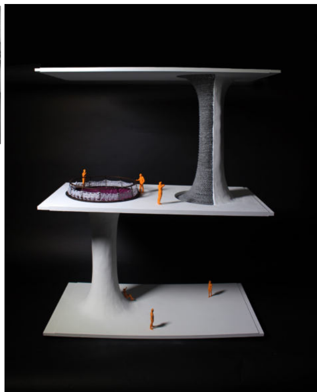
Image 06: Knitted formwork, structural cast Timber, knitted columns, cyanoacrylate, plasterboard adhesive
