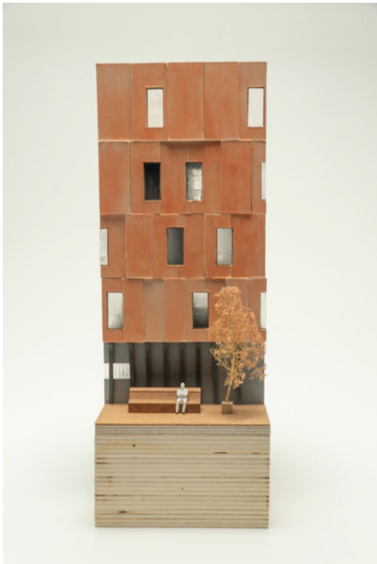
Image 05: Corner model Final Iteration 1:50 Scale 4, 6mm MDF sheet Non-stained plywood sheet (public space) Stained plywood sheet (private space) mahogany furniture Cork sheet (ancillary spaces + ground materials)
