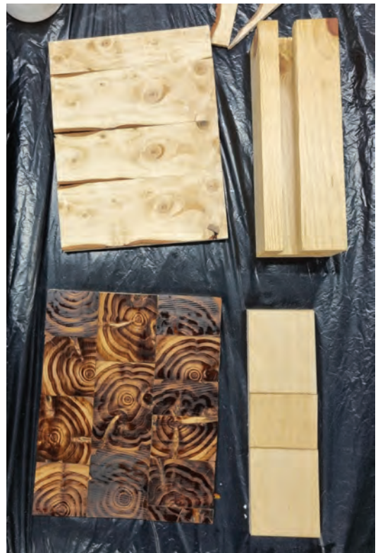
Image 6 1.5 Tactile Detail, process picture. Pieces were laid out to be sanded then varnished. Floor pieces were interlocked and the grain mixed up to create an interesting pattern.
