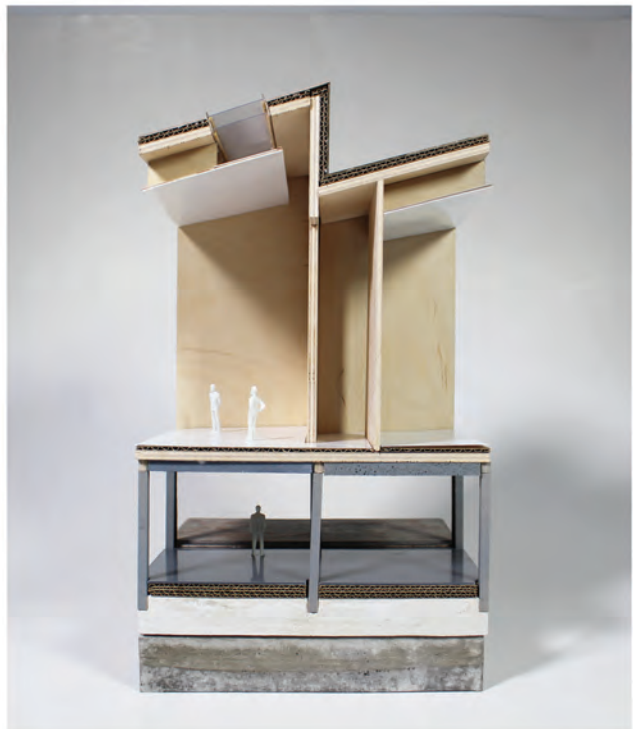
Image 2 1.50 Sectional Model, interior view. The image shows the nature of the interior gallery space, paying particular attention to the continuation of the thermal line along the section cut, and the skylight detail.
