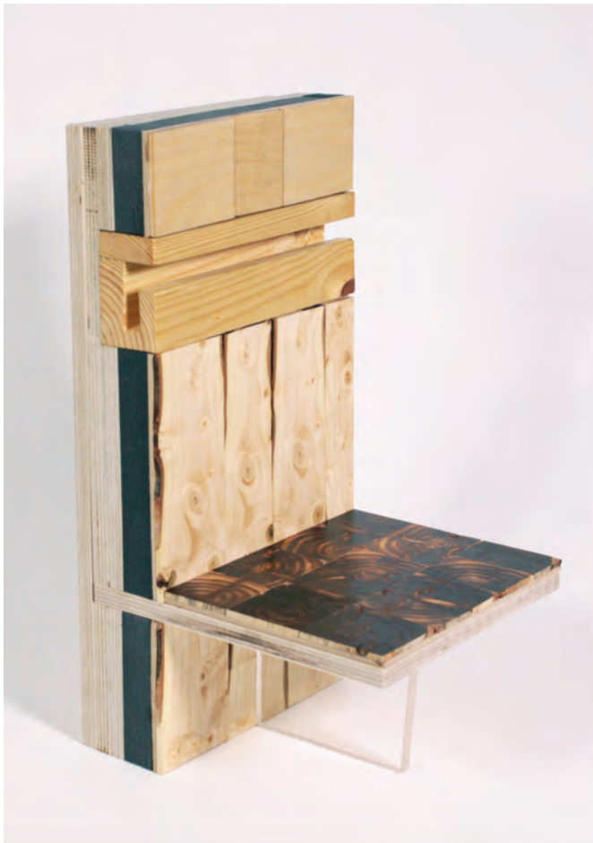
Image 5 1.5 Tactile Detail, overall view. Attention was paid to demonstrating how the handrail fits seamlessly into the wall using the section cut. I have taken advantage of the aesthetic qualities of the two directions of grain in the pine wood.
