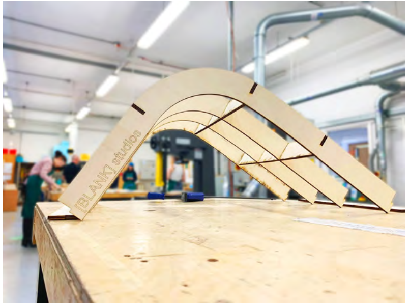
Image 03: Seat structure, cut with CAM, assembled in wood workshop (process)
