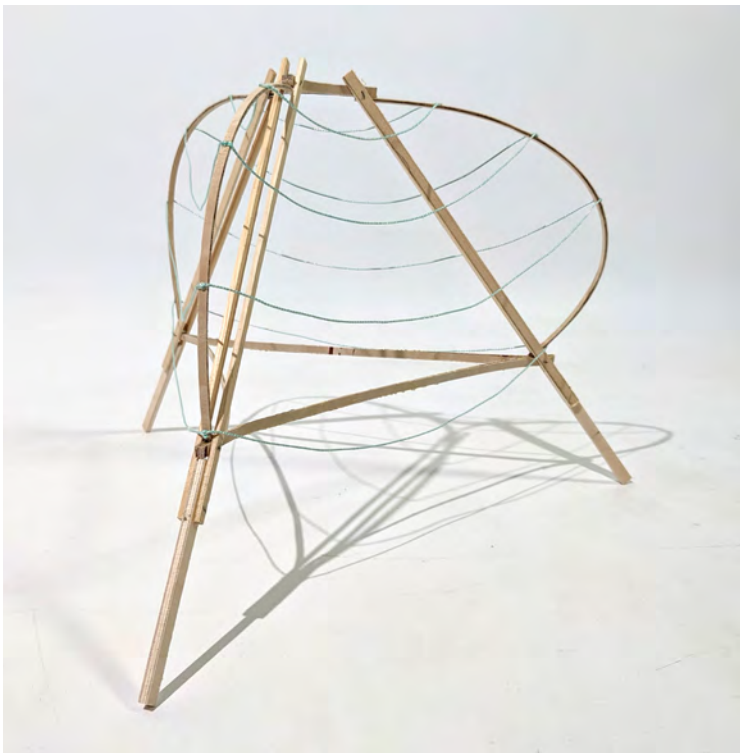
Image 02: 1:10 Structural Model - Plywood Strips, timber sticks, steel wire "bolts" (to allow movement at joints)
