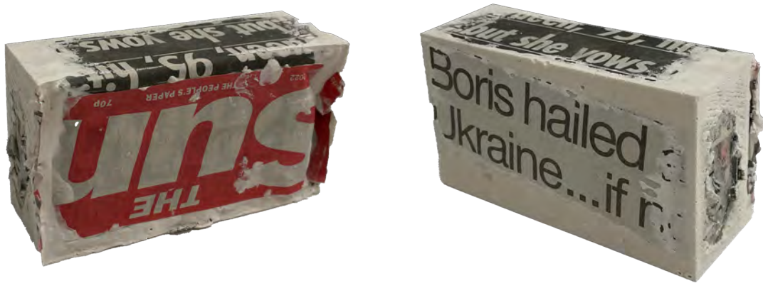
Image 11: 1:1 Models of papercrete bricks which were used using recycled newspapers which would become a tool to rebuild the new spaces for protestors
