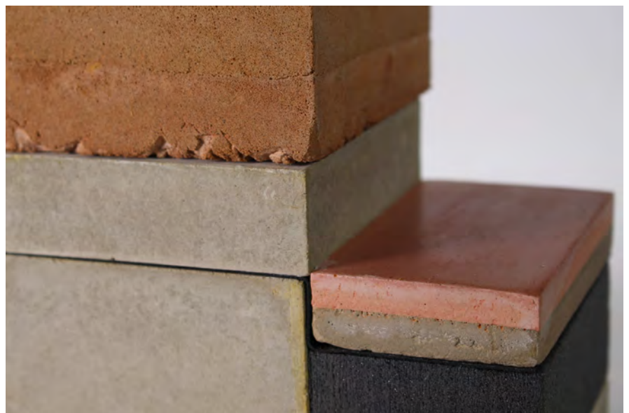
Image 01 [left]: The acrylic sheet etched by hand Image 02 [below]: The view of the model consisting of multiple layers of cast elements. The presented view shows the interior floor layers and the wall upstand
