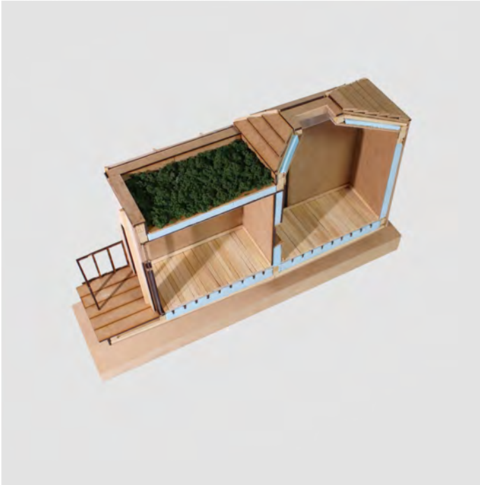
Image 06: Roof Treatment, internal flooring and outdoor decking
