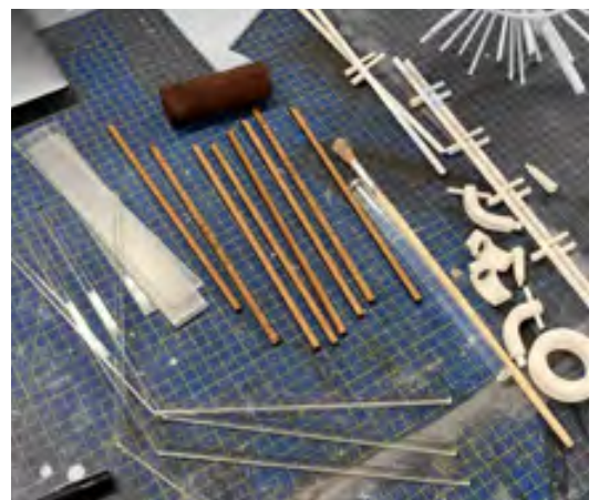
Image 5: The laser cut and 3D printer produce different parts of the model. There are several iterations for improving the precision and design of the model during the model assembly.
