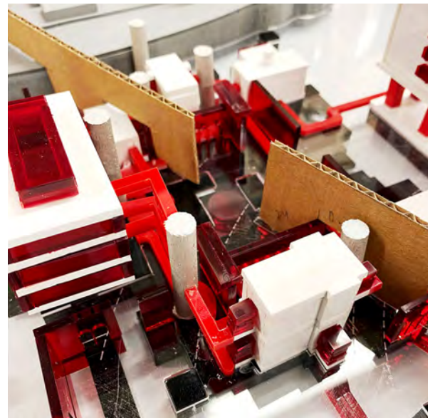
Image 05: The Experiment- using cardboard to get the right heights and widths before laser-cut.
