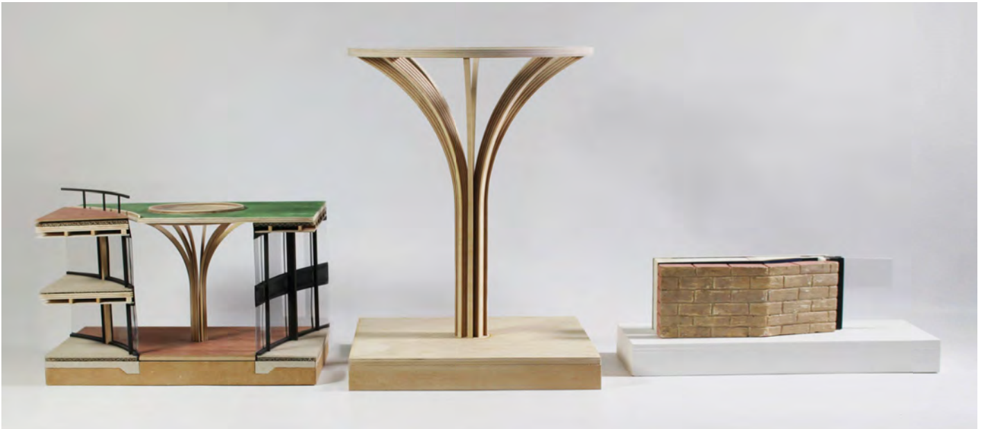
Image 01: The three final models made to communicate the design: (left to right) 1:50 corner detail, 1:20 column detail, and 1:5 handshake detail.
