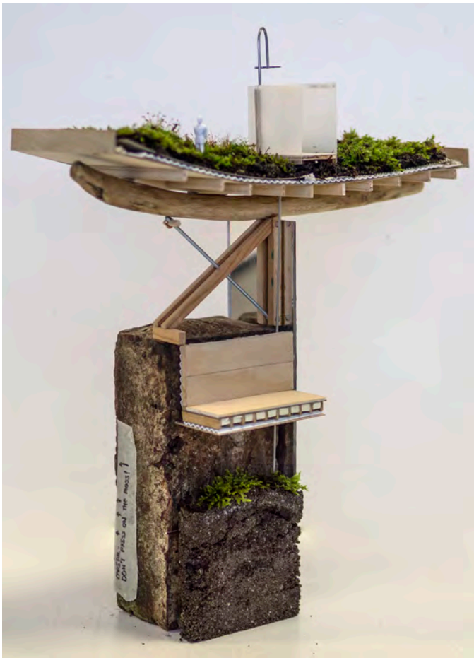
Image 03 : Moss roof house retrofit The moss roofs are the basis for flood-resilient, low-carbon house retrofits. Oak heartwood integrated to the roof trusses is a creative way to reclaim trees felled in the wake of the tunnel construction. The roof includes metal nettings that double as electrodes for a biophotovoltaics system, and a substrate (charcoal, sphagnum moss, sand, soil) suitable for mosses to thrive.
