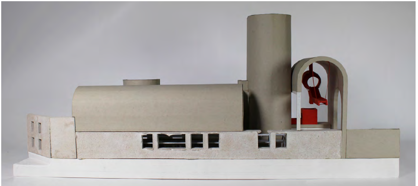
Image 04: Back of final section model, highlighting existing (jesmonite) vs new structure (recycled paper)
