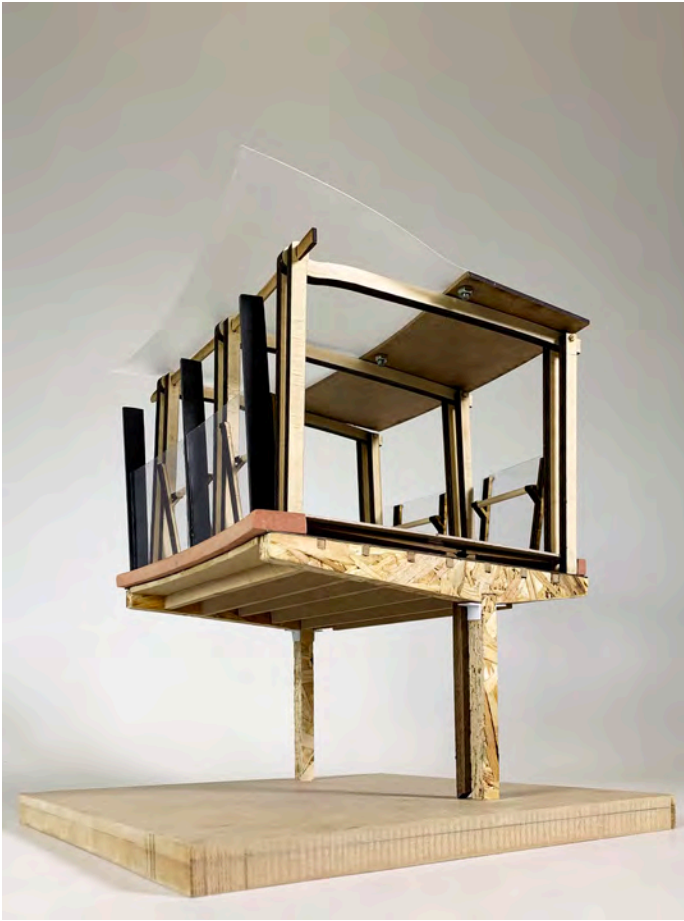
Image 04: Wooden Joinery of the Joist and Beams
