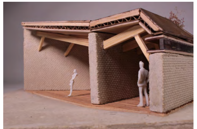
Image 05: 1:50 Section model, eye view showing the change in ceiling height
