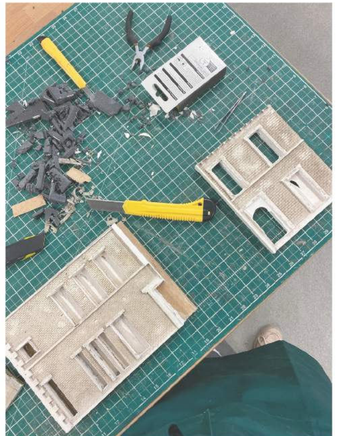
Image 02: Cleaning the plaster after drying.
