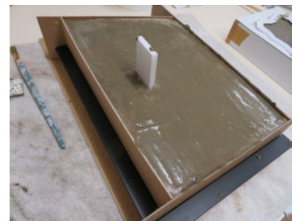
Image 05: Pouring the concrete.
