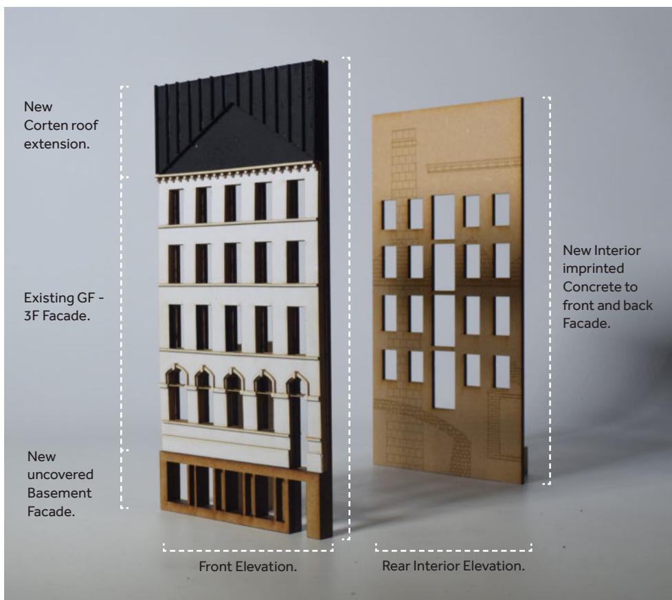
Image 3 - 1.100 Interior and Exterior Facade Model (MDF, Card).
