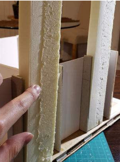
Image 09: Modelling process - applying insulation (polyurethane foam block)
