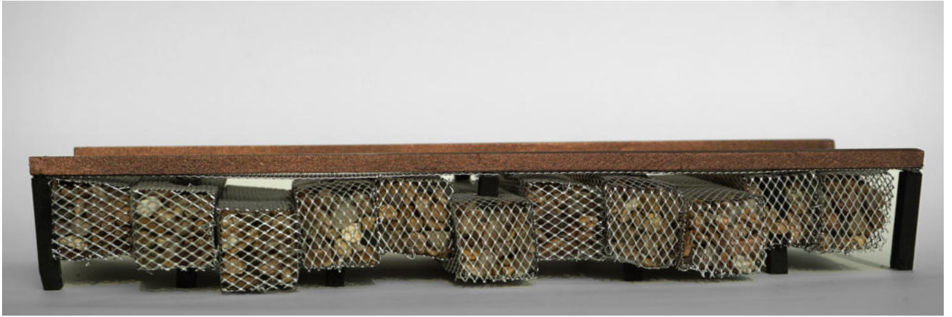
Image 04: Model front elevation showing the water outflows created by the gabion arrangement
