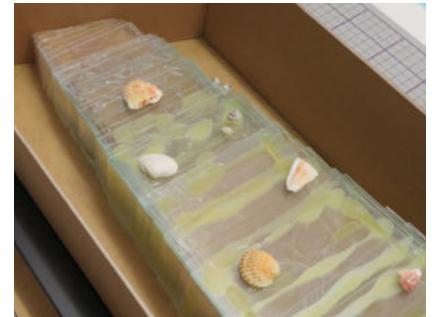
Image 04: Layering of Perspex to create the mould.
