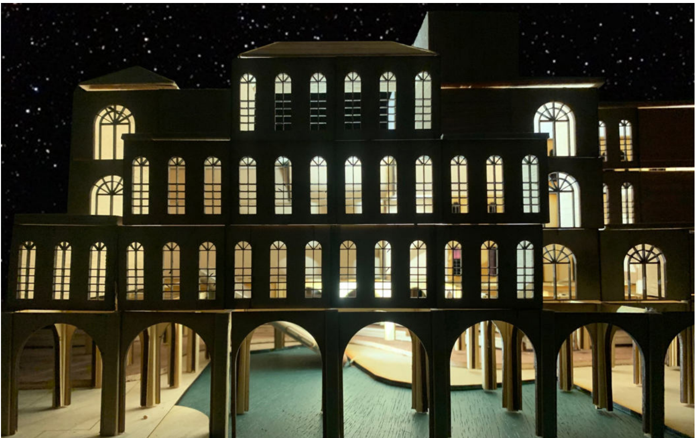
Image 01: 1:100 Site Model of Reeds - balsa wood (for roof structure and walls, plywood (site and walls with windows) and acrylic paint (lake on site).
