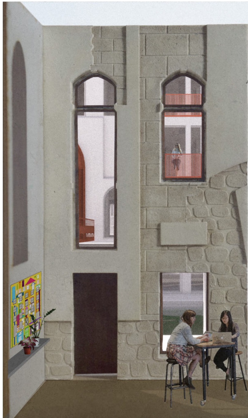
Image 4 - Looking to the interior imprinted facade. Rubble build up of the culvert and ashlar finish of the contextual façades imprinted in plaster to represent a concrete finish.
