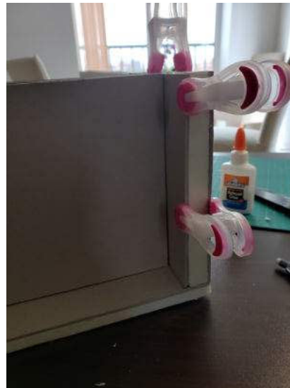
Image 10: Modelling process - Using laundry clips to secure glued sheathing board (grey mount board)
