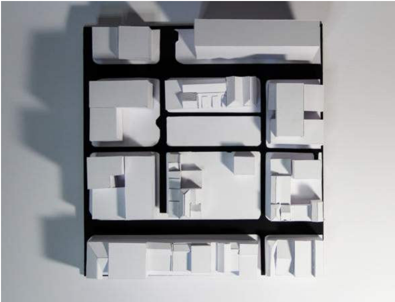
Image 02: The roofs of the surrounding had to be carefully detailed to see the light effects on the site.
