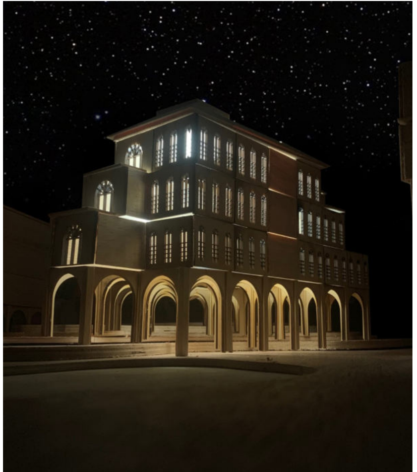
Image 03: 1:100 External view of Leve - soft plywood (arches), pine dowels (columns), hard plywood (site) and thin balsa sheets (floor above arches), thick balsa (walls without windows). The arches range from 40- 60mm high dependant on where it is situated on the landscape.
