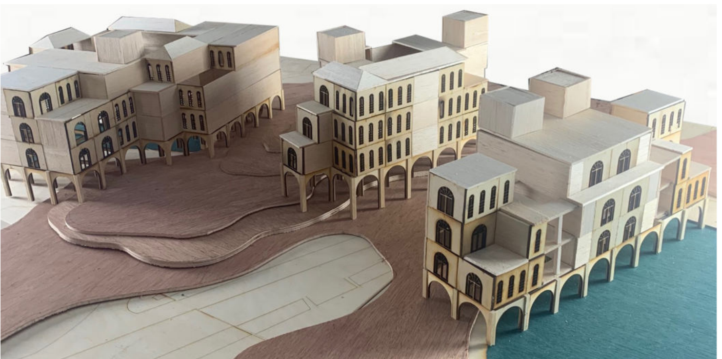
Image 05: 1:100 Site Model, Isometric South West View of Reeds (left), Leve (middle), Fallofelde (right) - balsa wood, softwood and hardwood plywood, pine dowels and acrylic paint.
