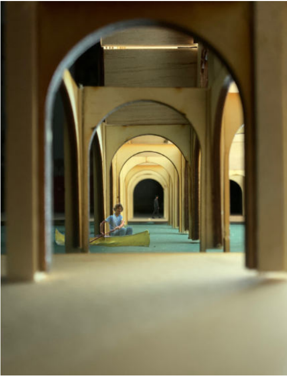
Image 02: 1:100 The building arches - soft plywood (arches), pine dowels (columns), hard plywood (site) and thin balsa sheets (floor above arches).
