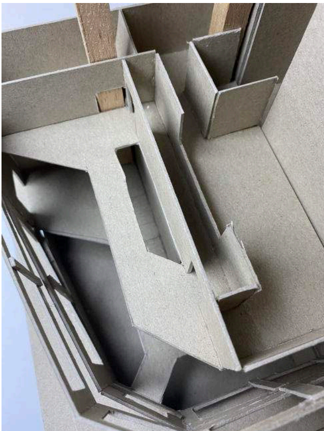
Image 01: Greyboard 1:100 developmental model with a modular design to understand verticals and floorplans.
