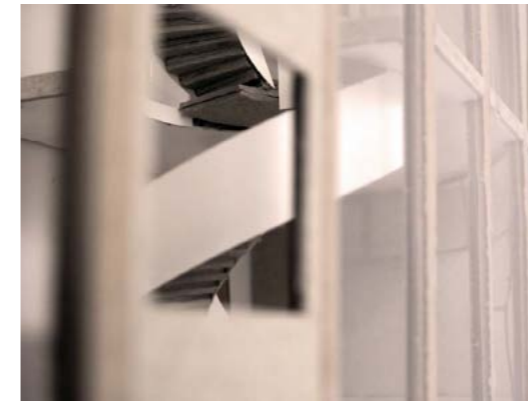
Image 04: Stair Detail - Greyboard, acrylic sheet, corrugated cardboard, catridge paper
