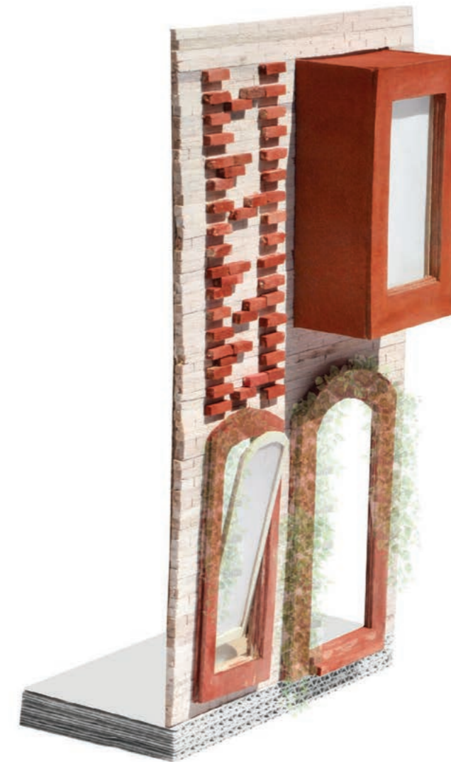
Image 05: 1:15 Façade section model showing ornament, ground floor pivoting window, house threshold and cantilevered reading space
