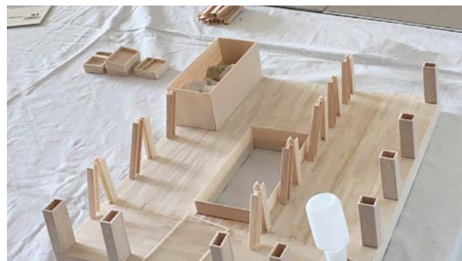
Image 02: I placed rocks inside the core to make the back of the model weigh more than the front, which allowed the cantilevers stand horizontally straight.
