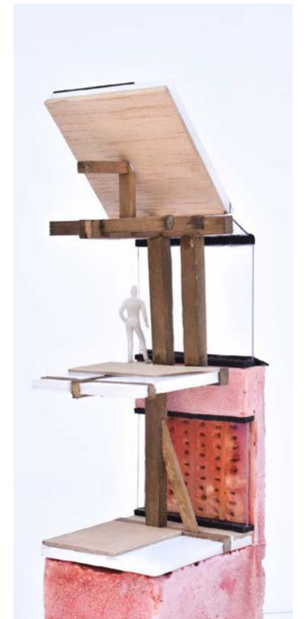
Image 04: Contrast between old timbers and new perforated brick.
