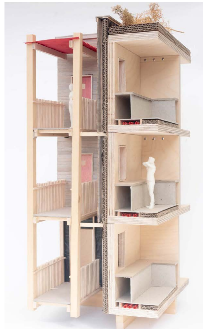
Image 05 + Image 6: 1:20 sectional detail model showing the construction of the wall to floor slab interfaces for three flats. External walkways leading to the entrance of separate flats highlight their relationship to the windows of the sectioned flats. Plywood was used to represent structural CLT and was manufactured in the workshop prior to lock down. The rest of the model was made at home using primarily a combination of corrugated card, balsa and grey board.
