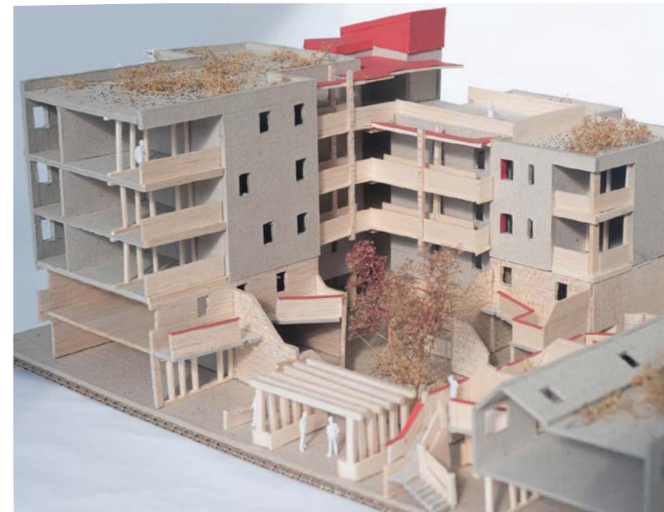
Image 03: 1:100 presentation model showing the communal centre and its relationship to the dwellings, their private gardens and the communal circulation for flats. Entirely handmade using varying thickness's of grey board and balsa, and red paper.
