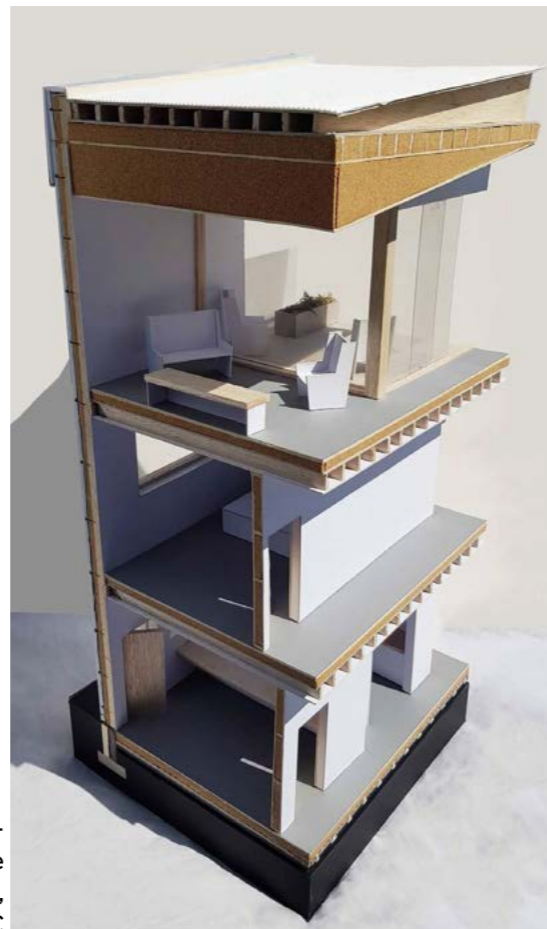
Image 02: Sectional Model - North and West face Foam core board, cork, balsa, mount board and PVC
