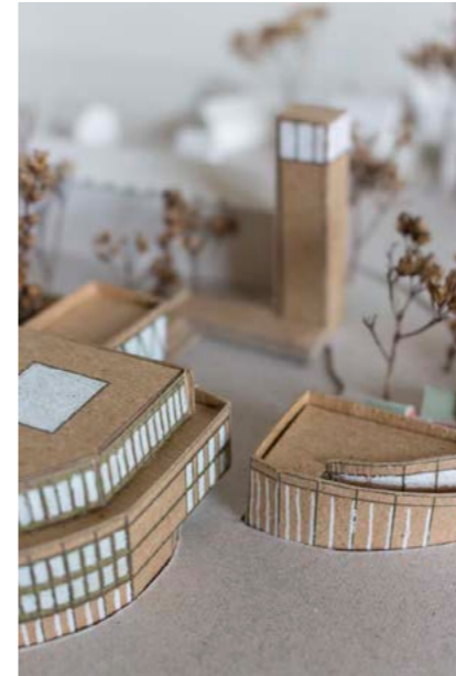
Image 04: A close-up of the proposed new buildings. Folded out of brown paper and hand painted with a pen.
