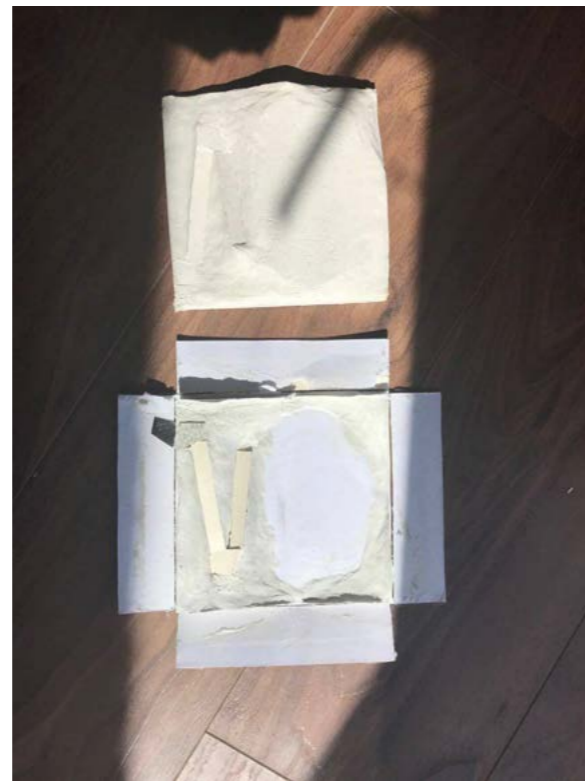
Image 02: Process: mountboard and plasticine mould with the plaster result.
