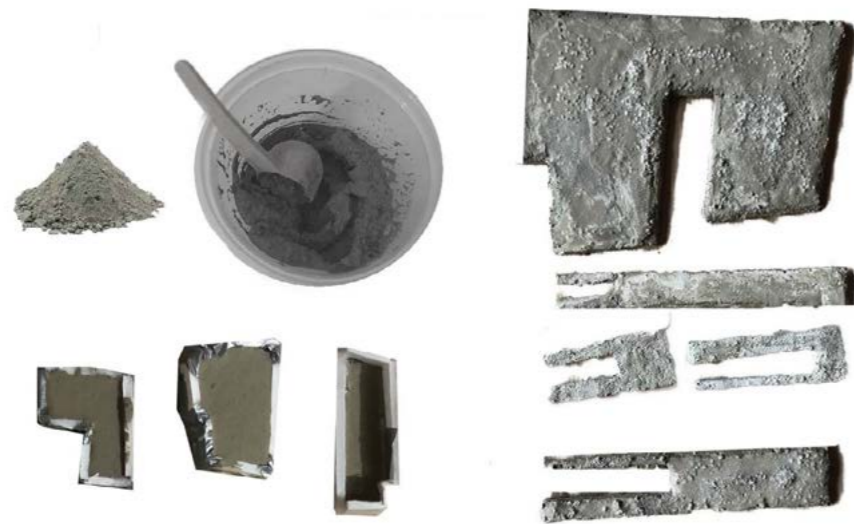
Image 01: Concrete Casting Process
