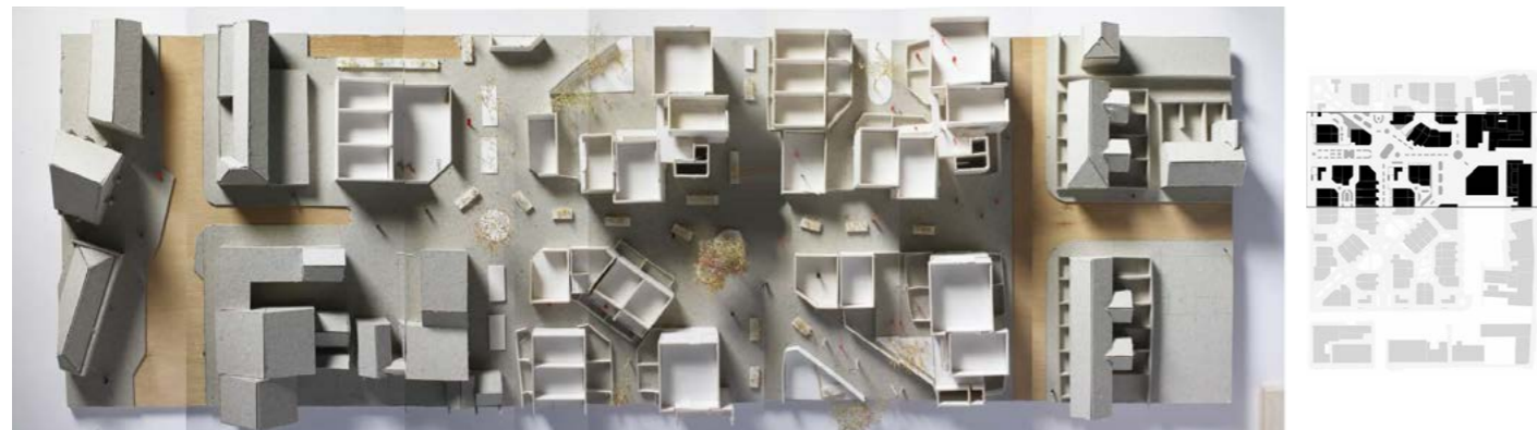
Image 01: 1:200 working model exploring the urban design of a portion of the larger masterplan. A plywood base was cut in the workshop. Hand cut grey-board was used for context, hand cut cartridge mount-board for the new build residential.
