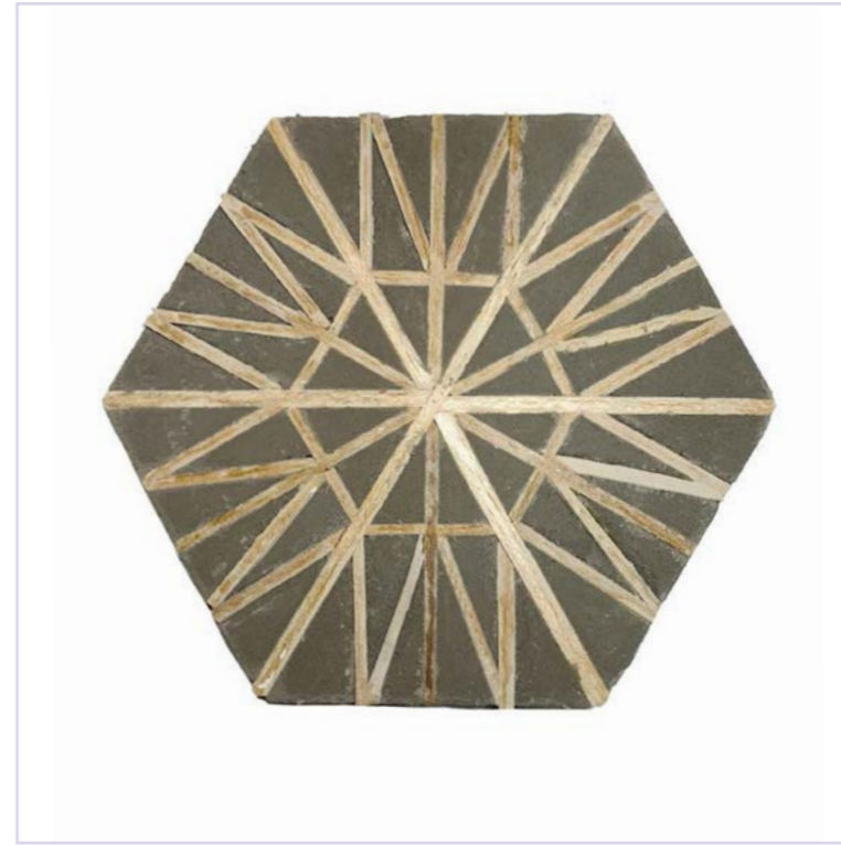
Image 04: Pavement detail model - Cast cement and balsa
